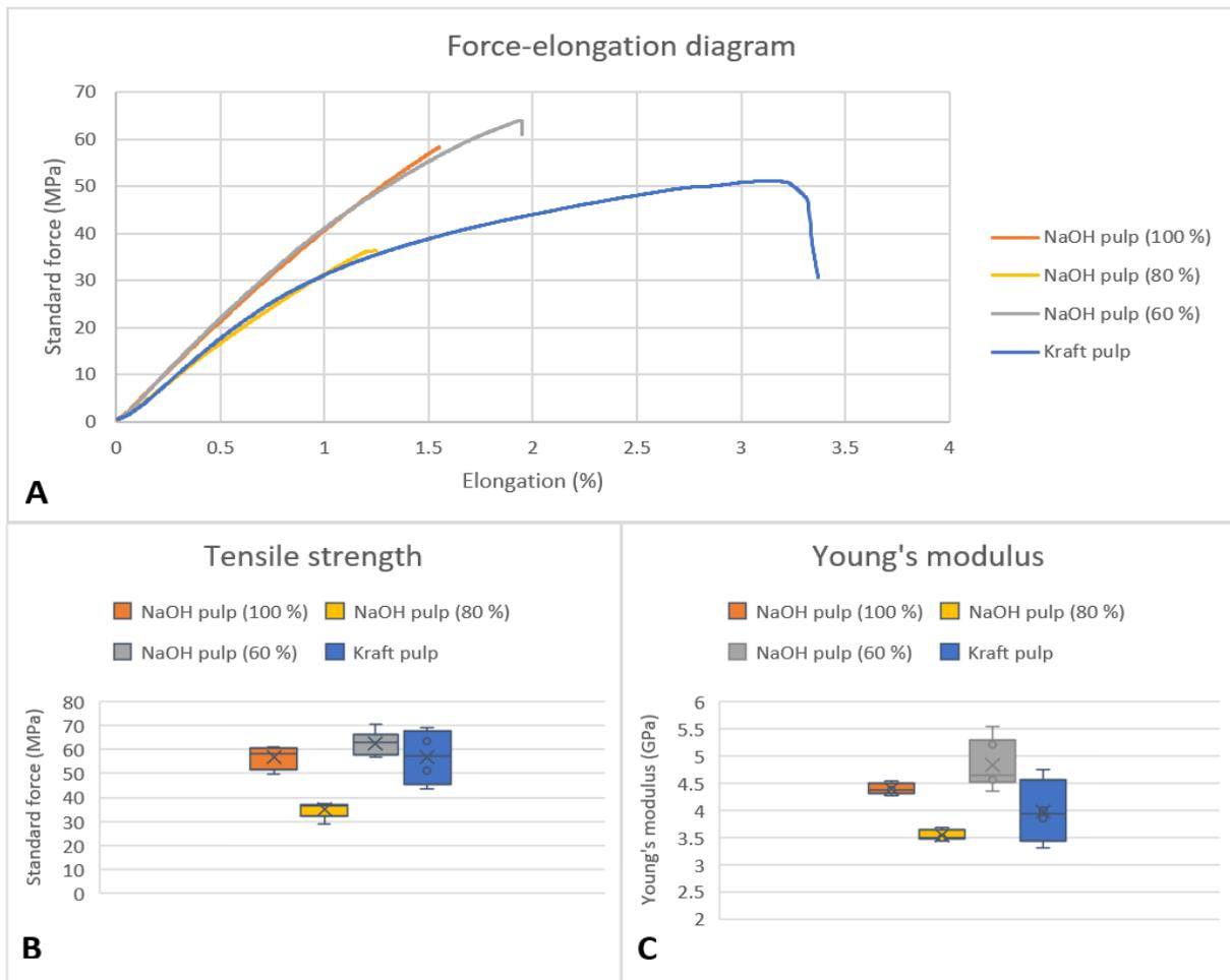
Figure 15: Various diagrams of 60, 80 and 100 wt% *M. spicatum* NaOH pulps with kraft pulp as reference; A: Typical force-elongation diagram; B: tensile strength box plots; C: young's modulus box plots.
