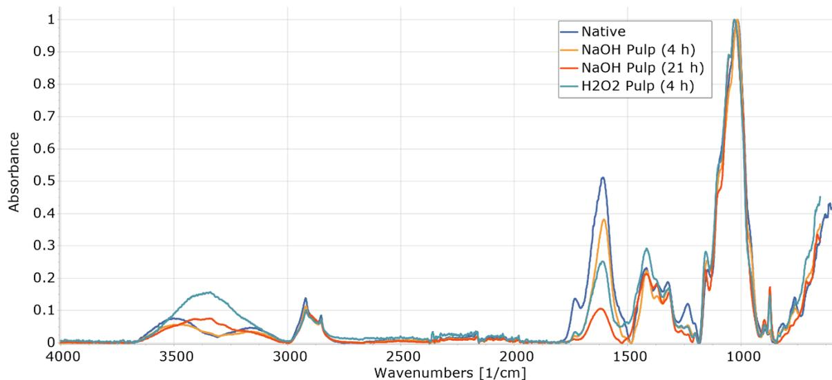
Figure 10: Comparison of the ATR-FTIR spectra of native *M. spicatum*, soda pulp (4 h and 21 h) and H<sub>2</sub>O<sub>2</sub> pulp (4 h).
