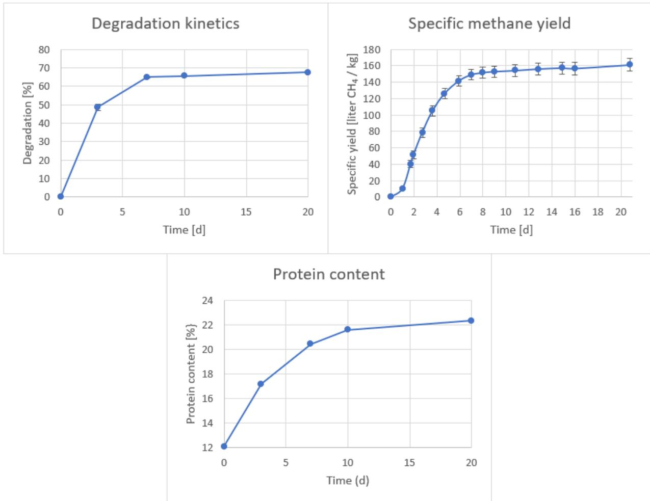
Figure 18: Several diagrams of the biogas experiment of *M. spicatum* over a period of 20 days: degradation kinetics (A), specific methane yield (B), protein content (C).
