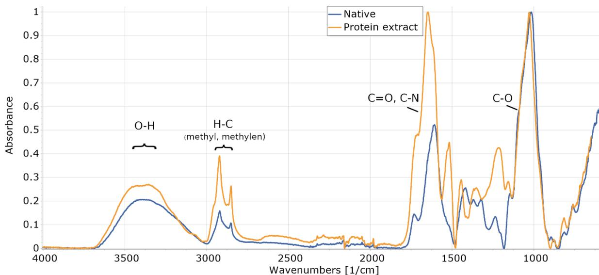
Figure 6: Comparison of ATR-FTIR spectra of native *M. spicatum* and the protein-rich fraction.
