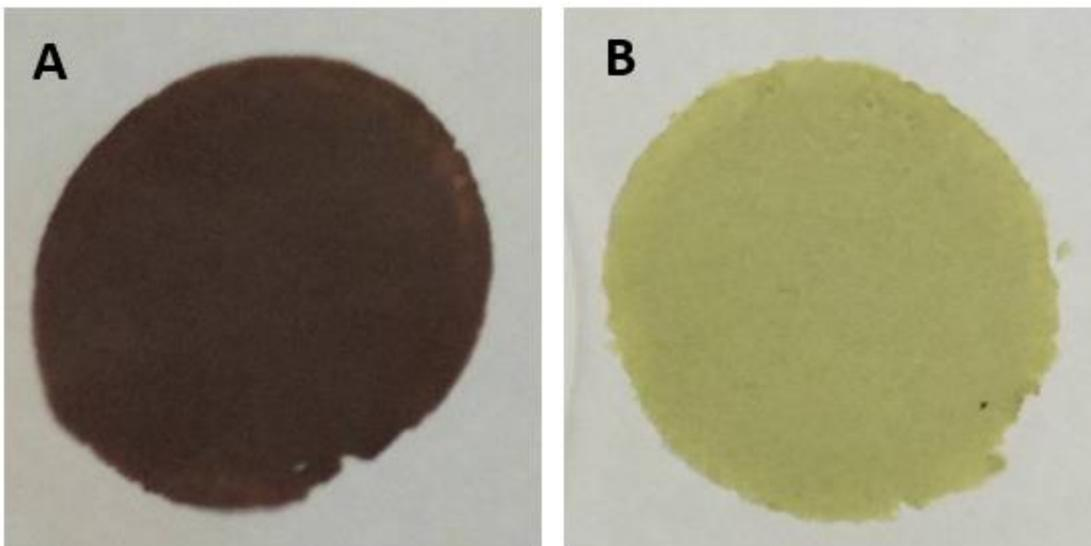
*Figure 12: Paper samples made purely from NaOH pulp (A) and from  $H_2O_2$  pulp (B).*
