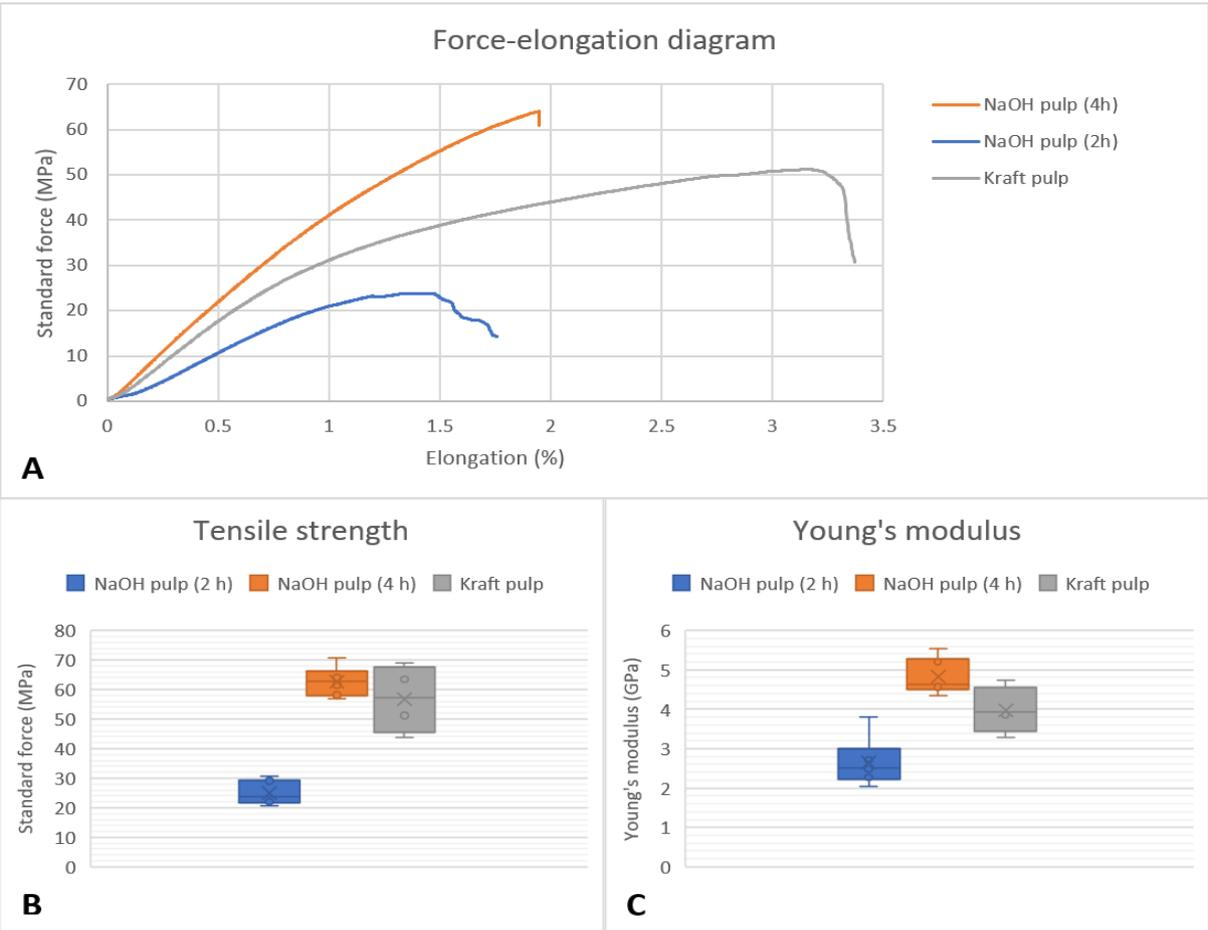
Figure 14: Various diagrams of 60 wt% *M. spicatum* NaOH pulps after 2 and 4 hours of pulping with kraft pulp as reference; A: Typical force-elongation diagram; B: tensile strength
