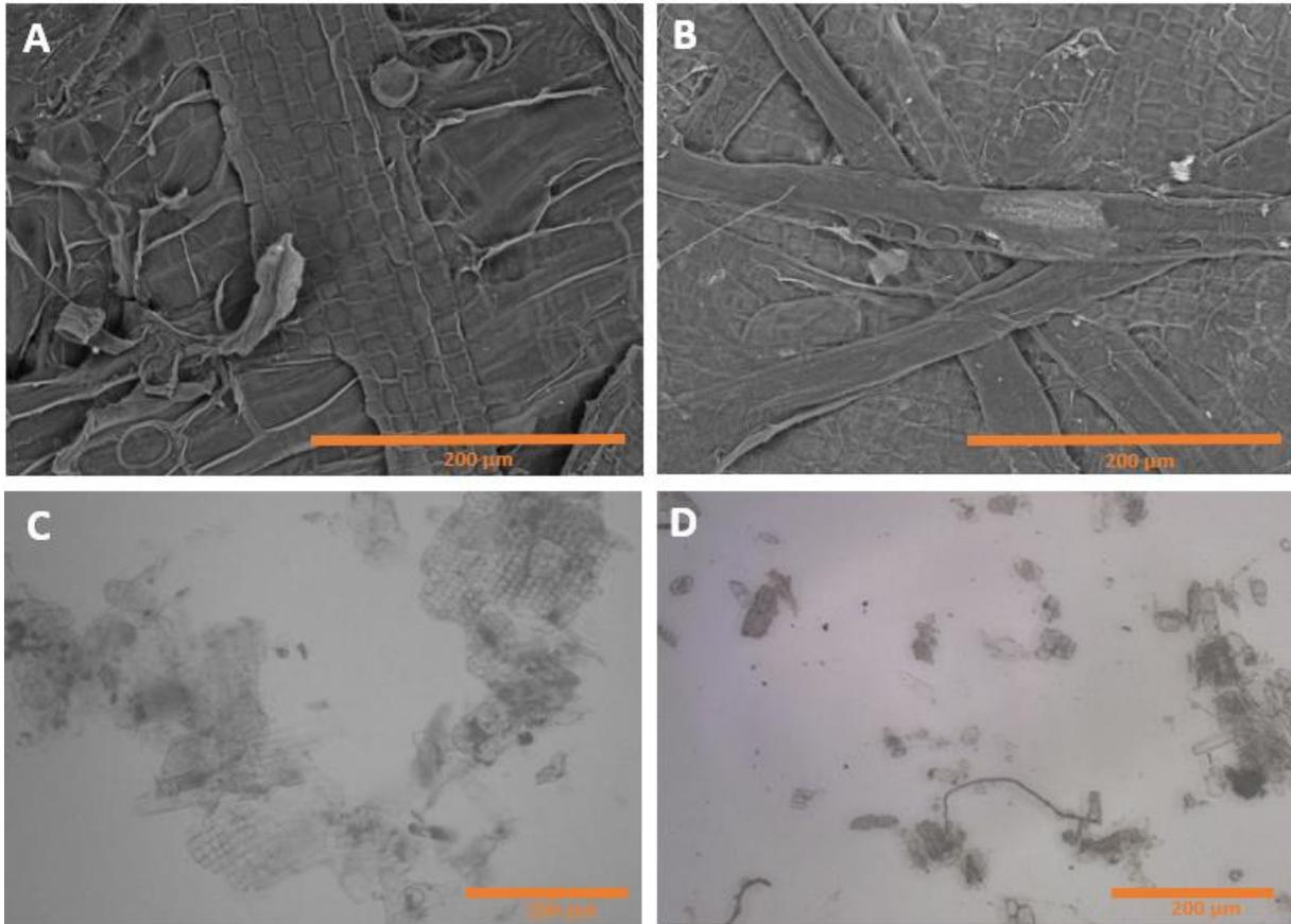
Figure 17: A+B: Blended paper made from 60 %  $H_2O_2$  pulp and 40 % kraft pulp, taken via SEM; papers made from pure NaOH pulp (C) and pure  $H_2O_2$  pulp (D), taken via light microscopy.
