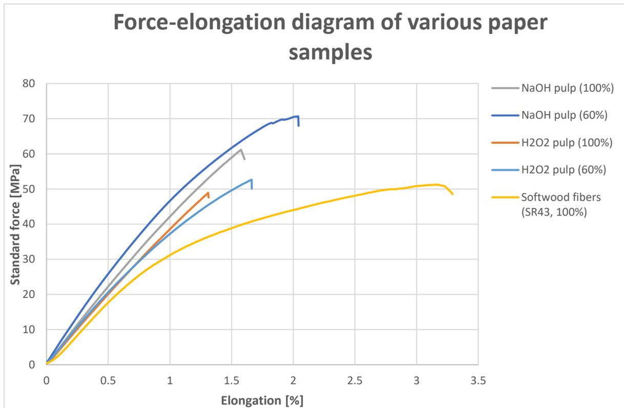
Figure 13: Typical tensile strength measurement results of paper samples made from various pulps and blends.
