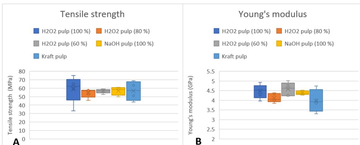
Figure 16: Tensile strength (A) and Young's modulus (B) box plots of 60, 80 and 100 wt% *M. spicatum* H<sub>2</sub>O<sub>2</sub> pulps with NaOH and kraft pulp as reference.
