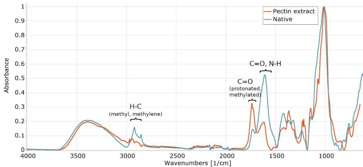
Figure 9: Comparison of ATR-FTIR analysis of pectin extract and native sample.
