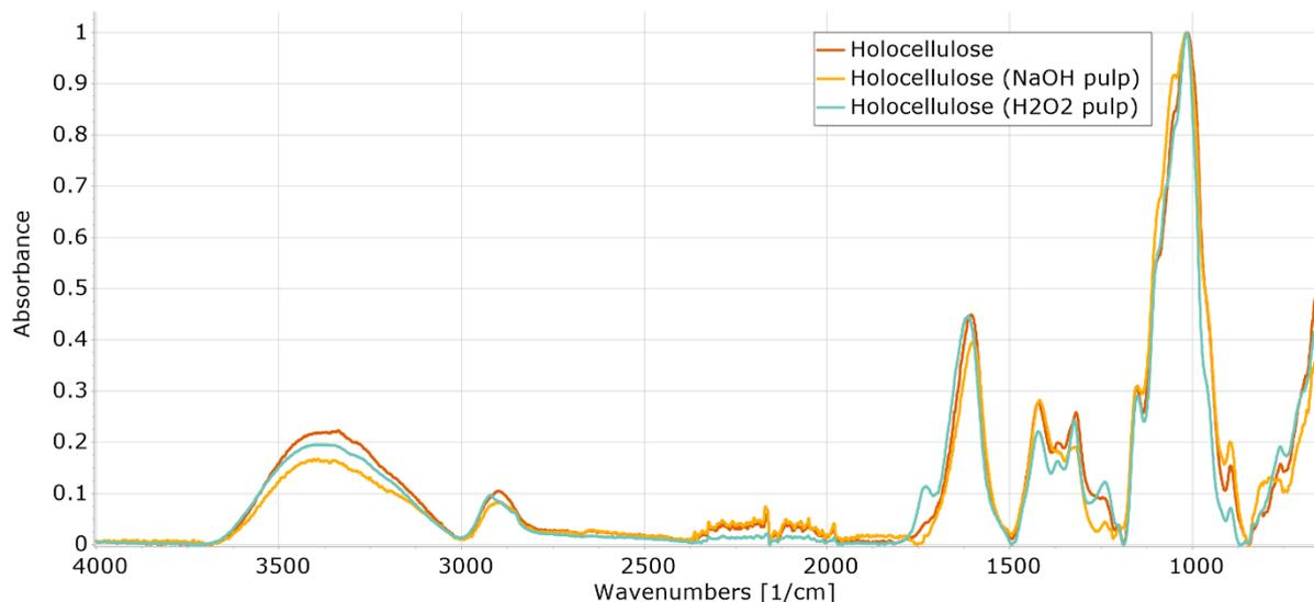
Figure 11: FTIR spectra of holocellulose from native material, NaOH and H<sub>2</sub>O<sub>2</sub> pulp.
