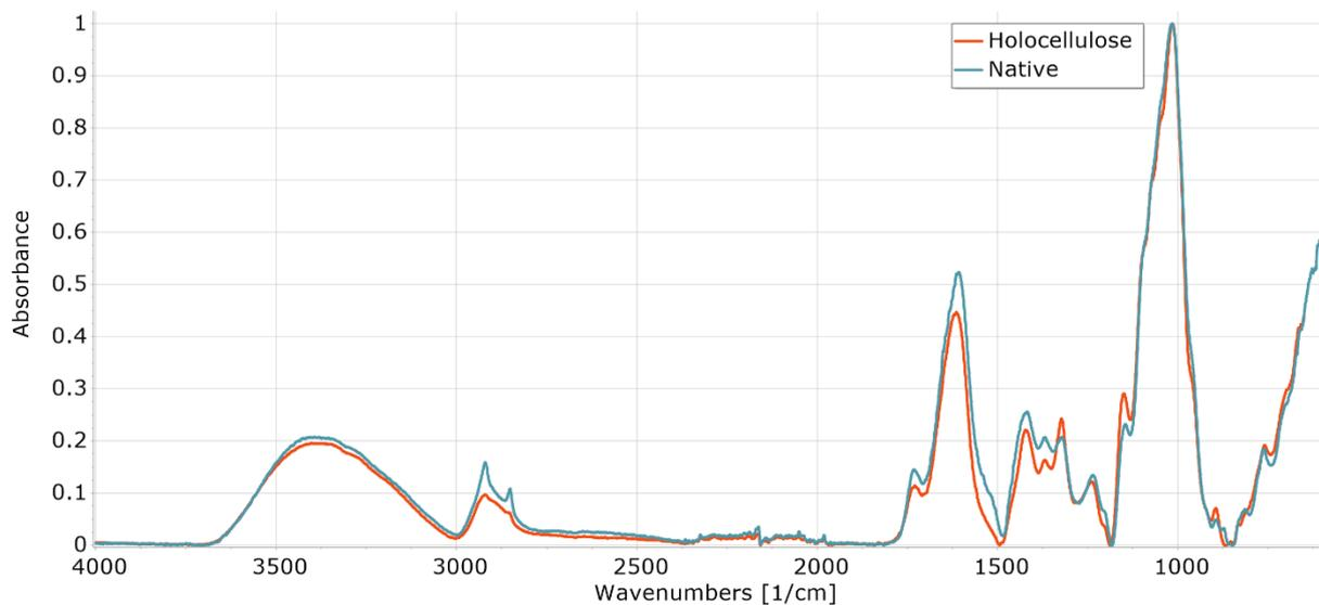
Figure 8: ATR-FTIR spectra comparison of holocellulose and native sample.
