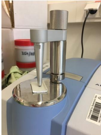
*Figure 5: Arrangement of the infrared analysis of a subsample for identifying the plastic type of the sample.*
