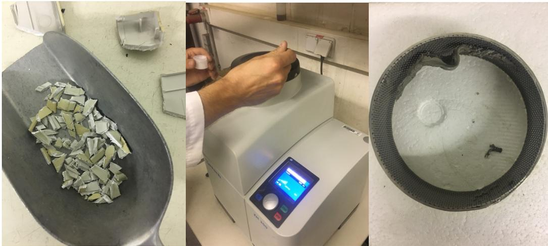
*Granulating procedure: (I) cut flat screen sample; (II) Pouring the sample in the centrifugal mill, milling; (III) distance sieve with melted flat screen sample (on the top of the image)*
