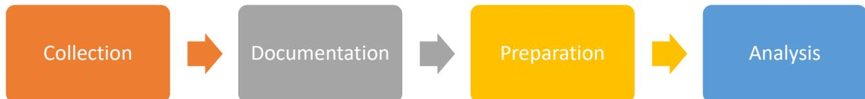
*Figure 4: Scheme of the sampling procedure. After collecting the devices from three different waste management facilities, they were documented. In a next step, subsamples have been extracted which were then used for the XRF measurement.*
