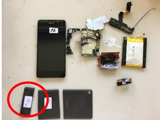
Figure 15: example of the dismantling and subsample preparation process
