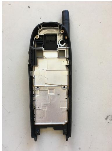
Figure 16: Unsuccessful preparation of a sample due to a metal-plastic housing
