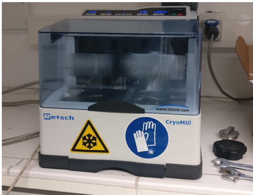
Figure 4: Used Retsch Cryomill to finely mill the samples via cryogenic grinding
