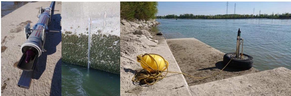
Figure 4: left receiver in plastic case ready to be deployed, middle: deployed receiver mounted to a wall, right: receiver with weight and buoy ready to be deployed
