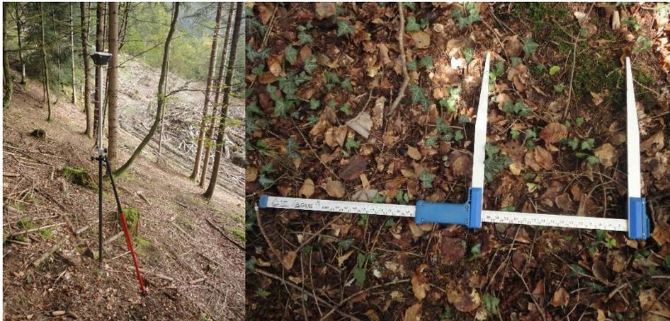
*Figure 28 a, b: Some fieldwork devices, on the left the GPS device and on the right the forest calliper used to measure tree diameter (Fotos: N. Guerrero Hue).*
