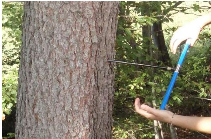
Figure 29: Coring a tree with the increment borer (Foto: N. Guerrero Hue).
