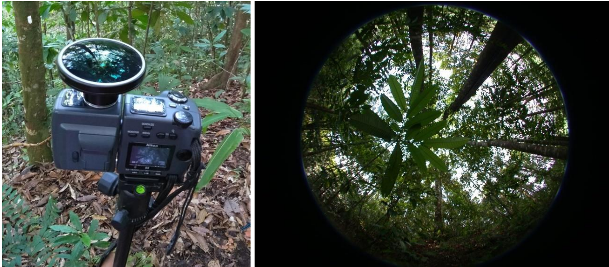
Figure 12: (a) Nikon Coolpix 995 camera setup with fisheye lens on monopod and (b) exemplary digital hemispherical photograph
