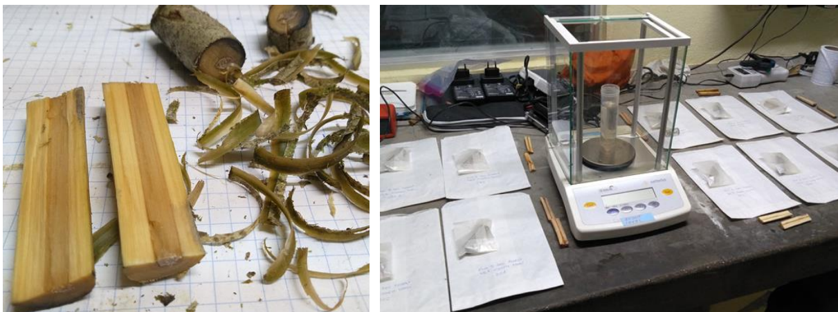
Figure 10: Processing of wood samples in laboratory including (a) splitting of branch samples and (b) volume measurements with water displacement method
