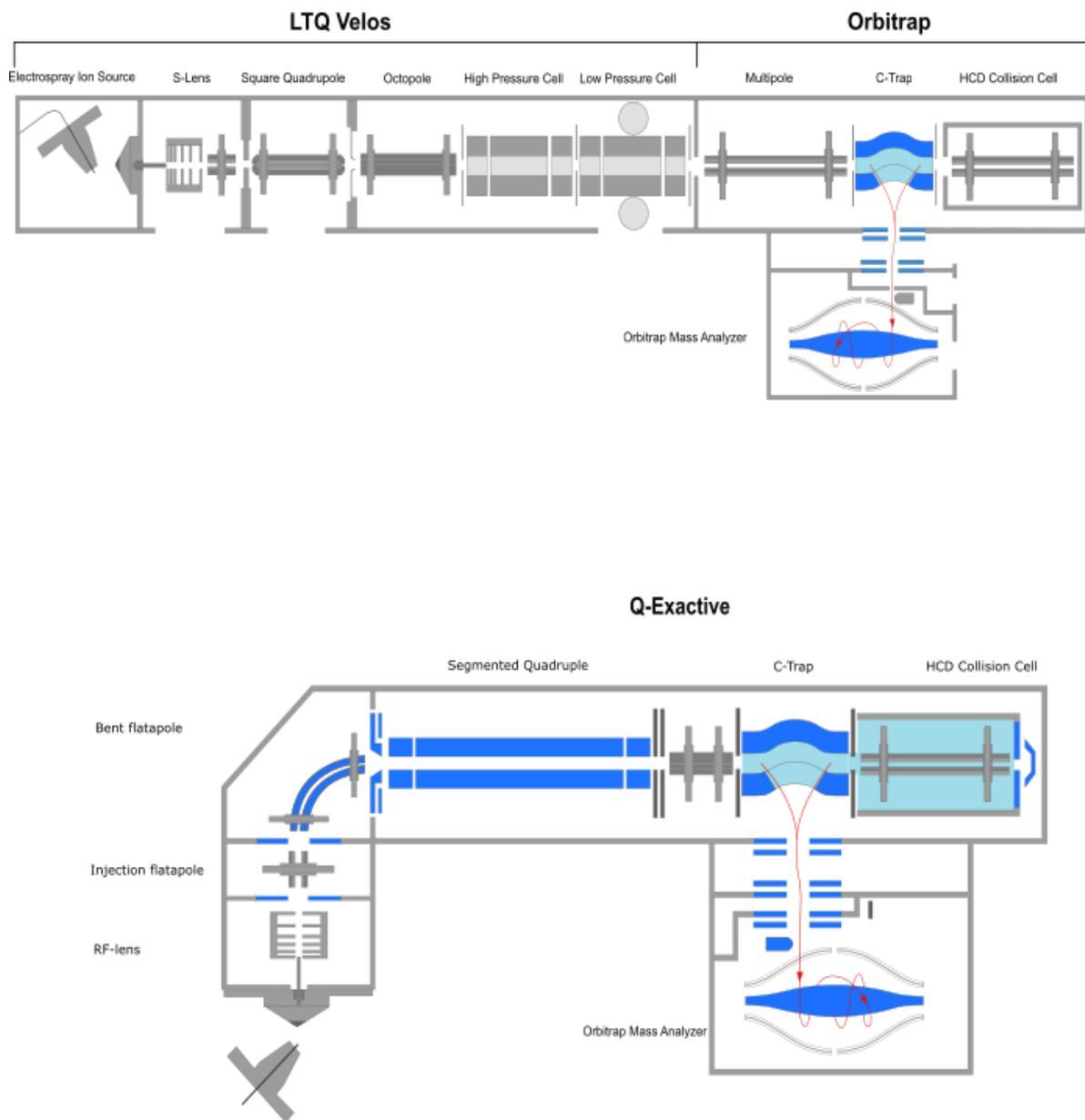
Figure 7 Schematic Diagram of LTQ Orbitrap Velos and Q-Exacte
