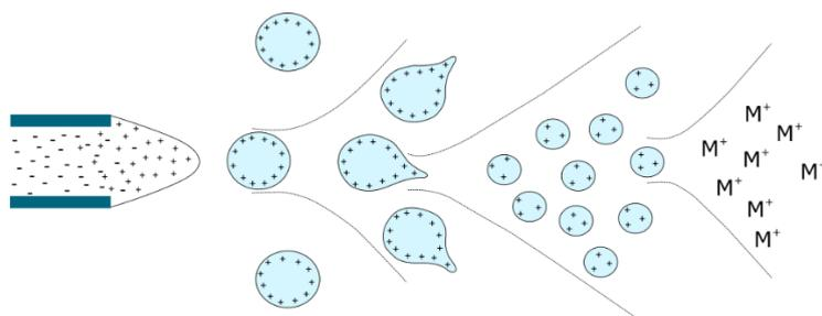
**Figure 4 Generation of ions by electrospray ionisation**
