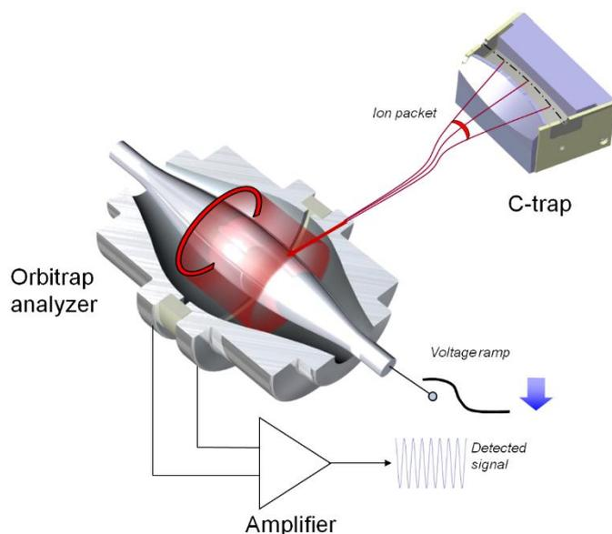
**Figure 5 Injection of ions into the Orbitrap mass analyser**
