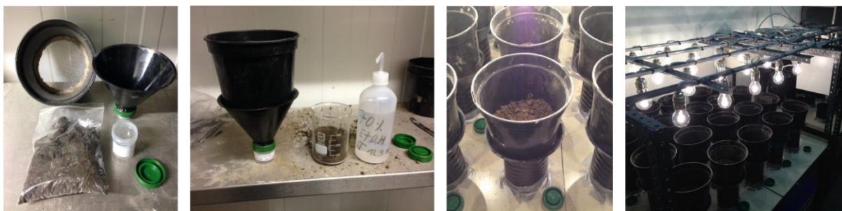
Fig. 2.4: Soil mesofauna extraction using the Berlese-Tullgren apparatus.
