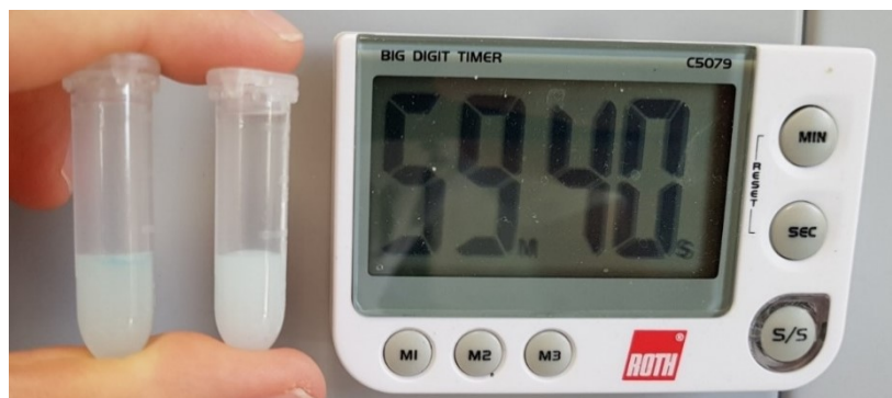
Figure 34: Photograph of optimized BCIP nanocapsules with 5000U/ml lysozyme (left reaction tube) and blank without lysozyme in the reaction mix (right reaction tube)
