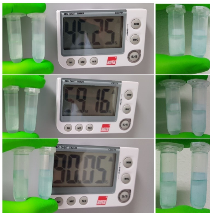
Figure 43: Color increase during incubation of the paper stripes with coupled AP, incubated with BCIP and lysozyme. Reaction tube on the left: Blank, reaction tube on the right: Sample.
