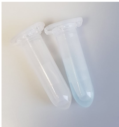
Figure 42: Color reaction of BCIP nanocapsules after overnight incubation with 10.000U/ml of Lysozyme
