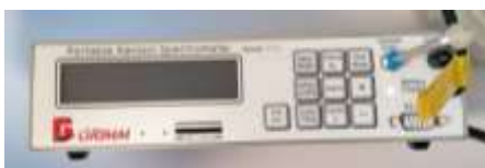
Figure 6 (Left): Optical particle counter – Portable Aerosol Spectrometer, GRIMM 11-C
