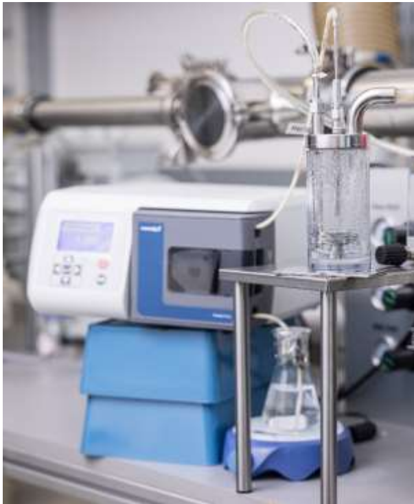
Figure 2: Transport of the starting suspension in the shake flask, standing on a magnetic stirrer, to the LSA by the usage of a peristaltic pump. The aerosolized particles in the LSA are then transported to the chamber by the compressed air, used for the aerosolization process.
