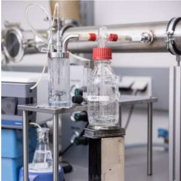
Figure 5: The Gas Washing Bottle (GWB) is directly connected to the LSA and the bioaerosol chamber. Therefore, the aerosolized particles are forwarded from the LSA into the buffer solution inside the GWB and then into the chamber.
