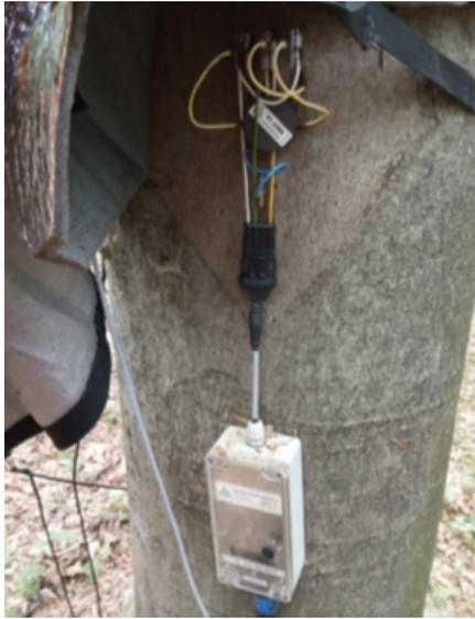
Figure 5: Sap flow measuring system on a beech tree on the DRAIN experiment in the LTER site Rosalia Forest Demonstraion Center (Figure credit: Kager, BOKU). To be seen are cables connecting the stainless electrodes (on top) with the sap flow sensor SF 81 (bottom) and the half removed weather shield.
