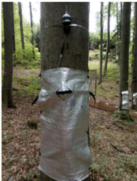
Figure 6: Insulating weather shield over a sap flow measuring system on a beech tree on the DRAIN experiment in the LTER site Rosalia Forest Demonstraion Center (Figure credit: Kager, BOKU)
