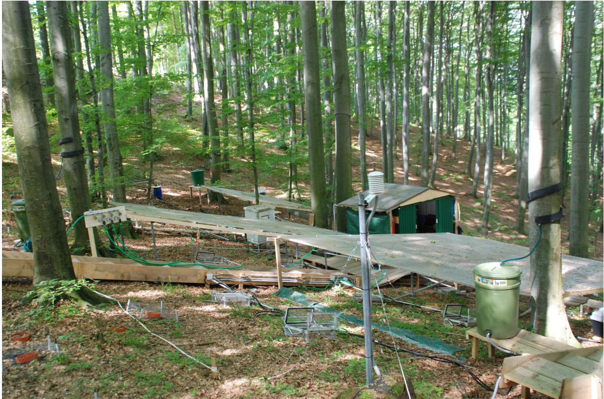
Figure 3: Picture of the DRAIN experiment in the LTER site Rosalia Forest Demonstration Center in 2019 (Figure credit: Institute of Soil Research, BOKU). Uphill sided of the transparent acrylic roofs the green foil of the trenches is visible
