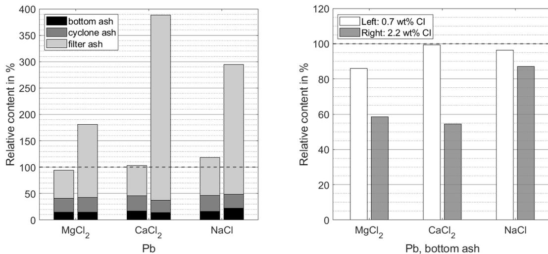
Figure 3.9: Pb content relative to benchmark experiment. Left figure: Pb content over all ash fractions. Right figure: Pb content in bottom ash
