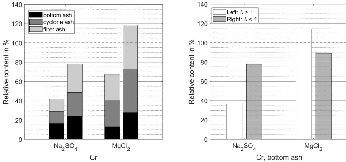
Figure 3.11: Cr content relative to benchmark experiment. Left figure: Cr content over all ash fractions. Right figure: Cr content in bottom ash
