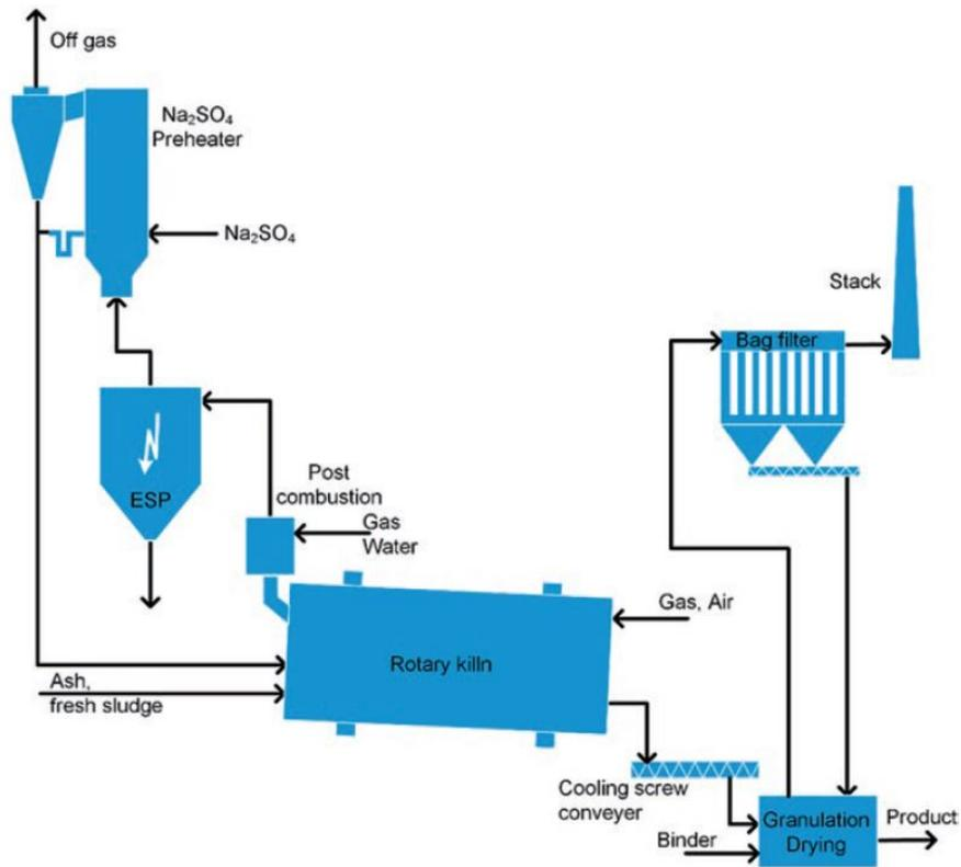
Figure 1.2: Flow chart of the AshDec process (Hermann and Schaaf, 2019)
