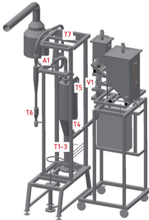
Figure 2.1: Photo of bubbling fluidised bed reactor and CAD drawing, modified after Langer (2020)
