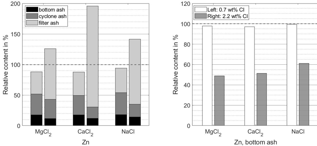
Figure 3.7: Zn content relative to benchmark experiment. Left figure: Zn content over all ash fractions. Right figure: Zn content in bottom ash
