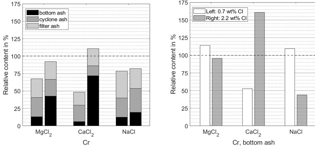
Figure 3.4: Cr content relative to benchmark experiment. Left figure: Cr content over all ash fractions. Right figure: Cr content in bottom ash
