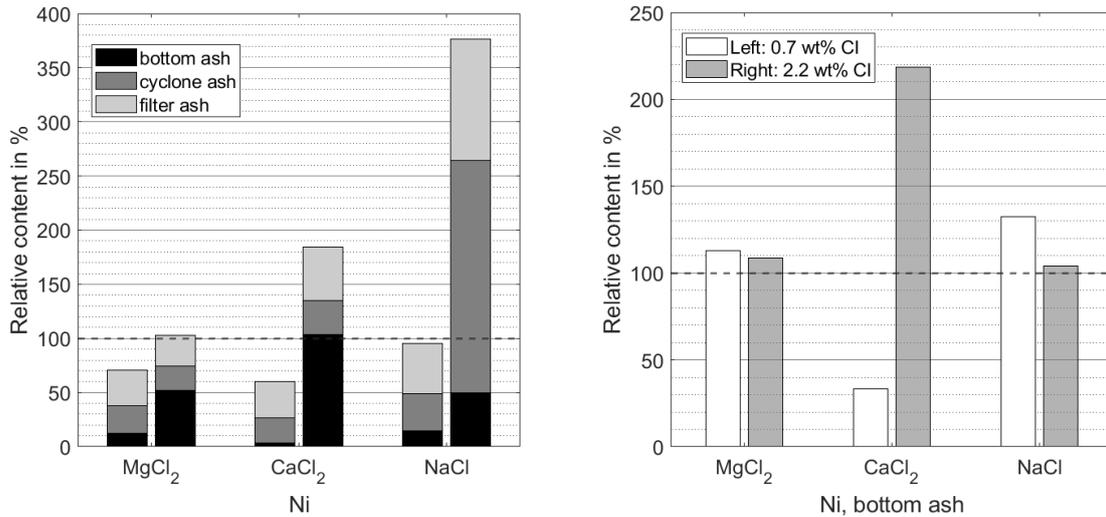
Figure 3.5: Ni content relative to benchmark experiment. Left figure: Ni content over all ash fractions. Right figure: Ni content in bottom ash
