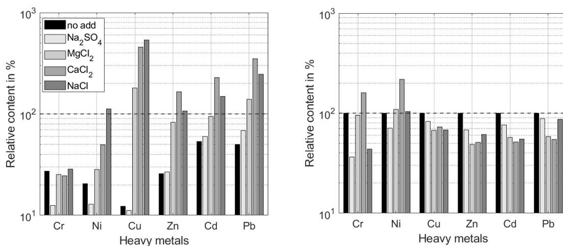
Figure 3.3: Left figure: Heavy metal content in filter ash fraction relative to total ash fractions of the no add experiment; Right figure: Heavy metal content in bottom ash fraction relative to the bottom ash fraction of the no add experiment
