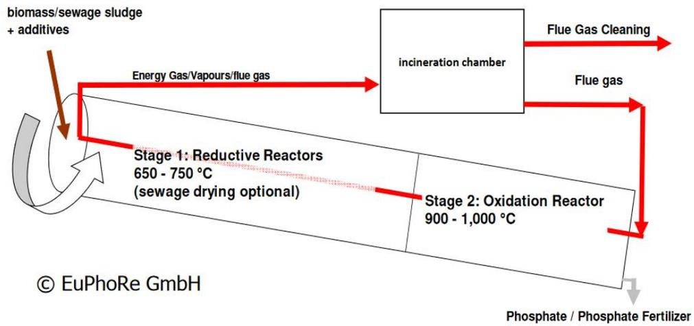
Figure 1.1: Flow chart of the EuPhoRe process (Hazard et al., 2018)
