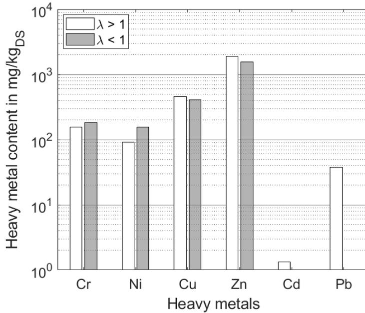
Figure 3.10: Comparison of heavy metal content in the bottom ash with  $\lambda > 1$  (left) and  $\lambda < 1$  (right) at 800 °C; bars not shown correspond to non-measurable values.
