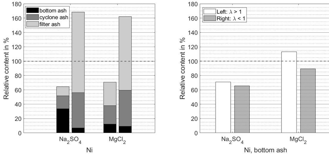
Figure 3.12: Ni content relative to benchmark experiment. Left figure: Ni content over all ash fractions. Right figure: Ni content in bottom ash
