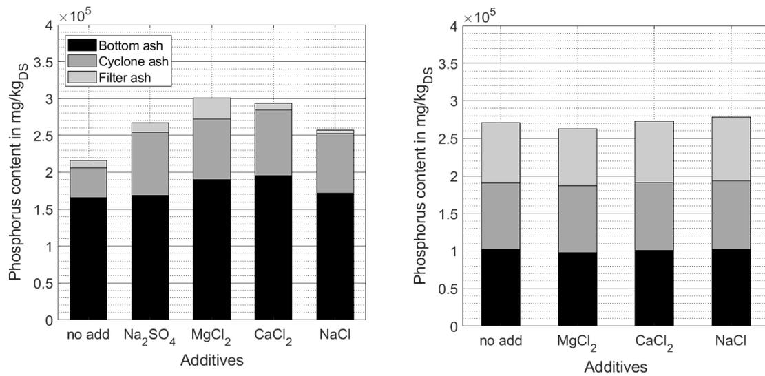
Figure 3.2: Phosphorus content in all ash fractions of sewage sludge 1 (left) and sewage sludge 2 (right) experiments.
