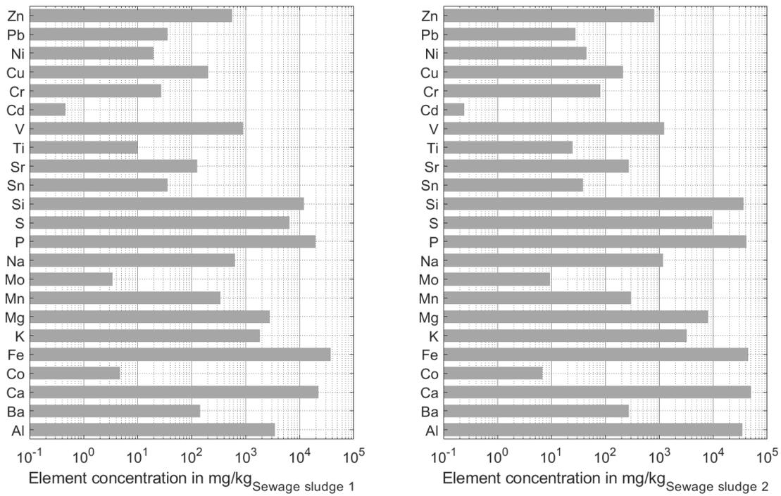
Figure 3.1: Composition of raw sewage sludge samples. Left figure: Sewage sludge 1. Right figure: Sewage sludge 2.
