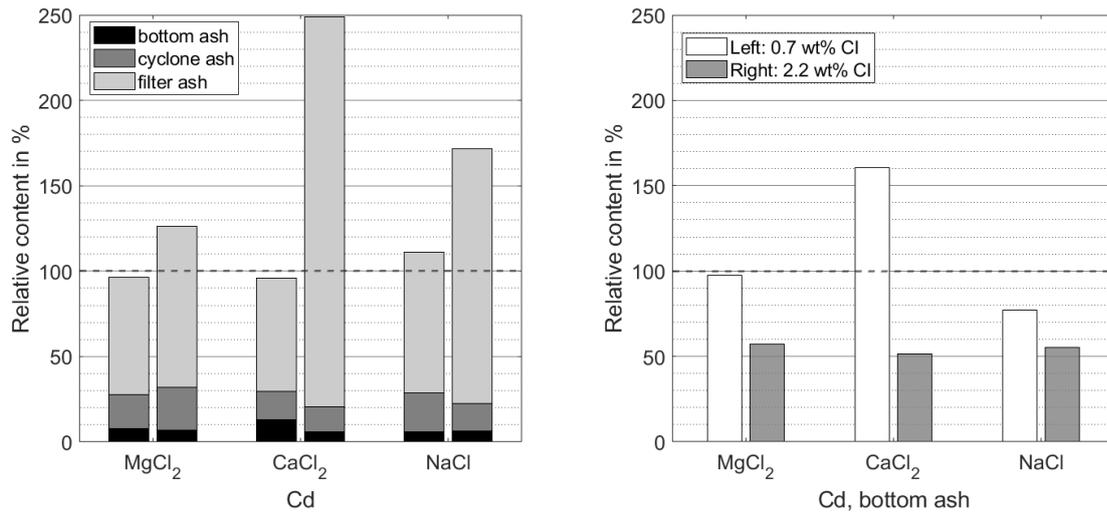
Figure 3.8: Cd content relative to benchmark experiment. Left figure: Cd content over all ash fractions. Right figure: Cd content in bottom ash
