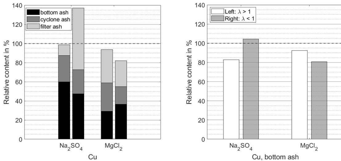
Figure 3.13: Cu content relative to benchmark experiment. Left figure: Cu content over all ash fractions. Right figure: Cu content in bottom ash
