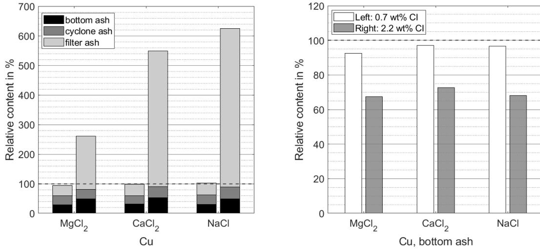
Figure 3.6: Cu content relative to benchmark experiment. Left figure: Cu content over all ash fractions. Right figure: Cu content in bottom ash
