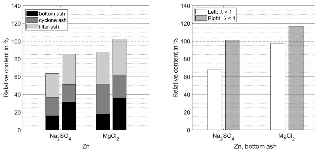
Figure 3.14: Zn content relative to benchmark experiment. Left figure: Zn content over all ash fractions. Right figure: Zn content in bottom ash
