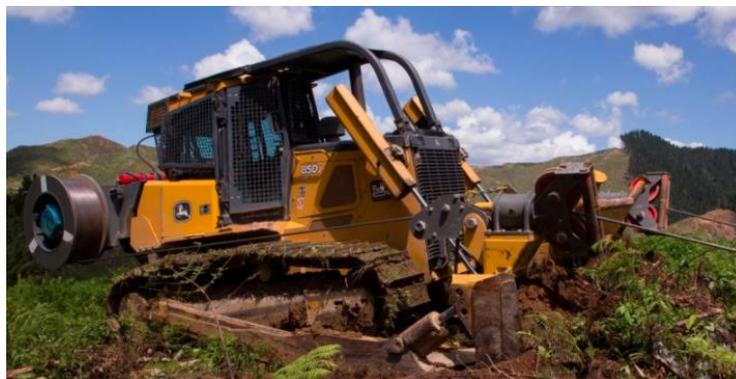
**Abbildung 6: ROB remote Operated Bulldozer (Rosewarne & May Limited, 2009)**
