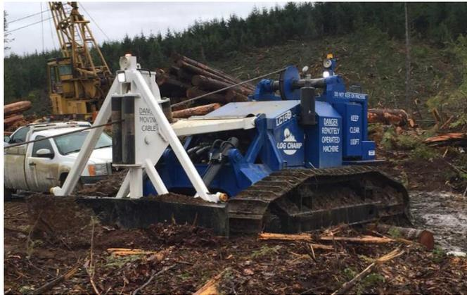
Abbildung 2: T-MAR LOG CHAMP 250 TRACTION WINCH (T-MAR INDUSTRIES LTD, 2019)
