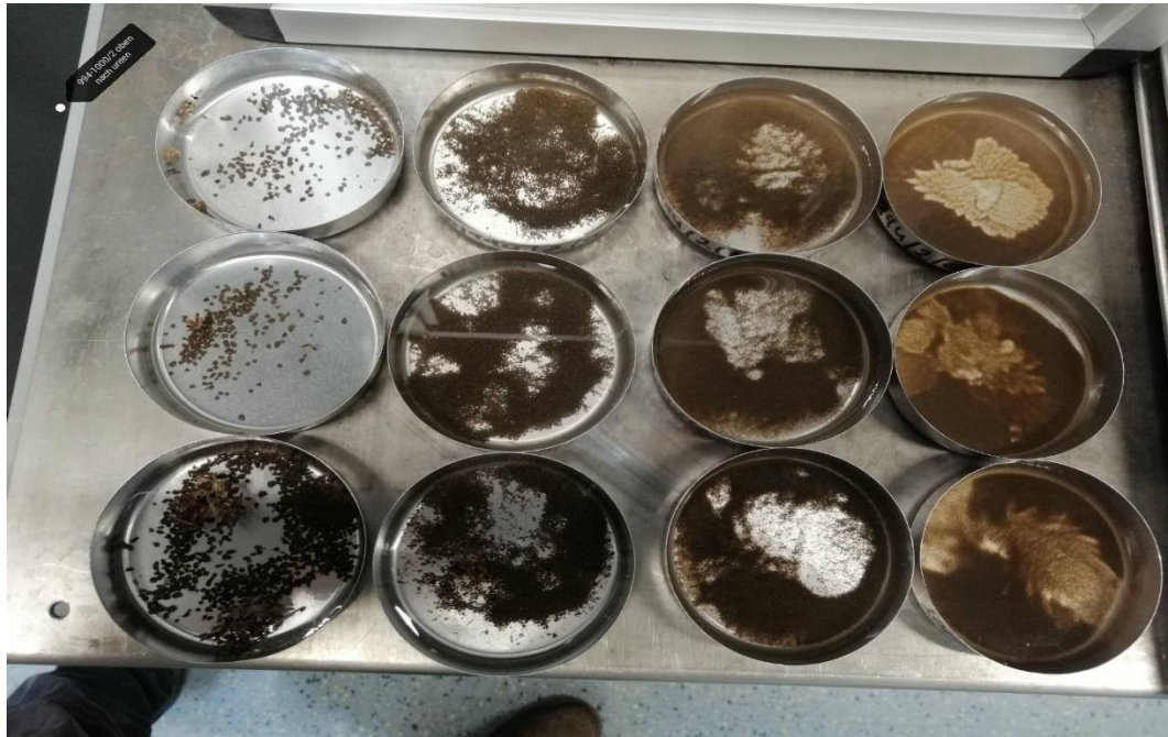
Figure Ap.2: Collected aggregate fractions from left to right: > 1000 \mu\text{m} - > 250 \mu\text{m} - > 63 \mu\text{m} - > 20 \mu\text{m} . From top to down: Pioneer – Standard – Reference of the heavy soil. Ultrasonic energy level, E1 = Spontaneous decay!
