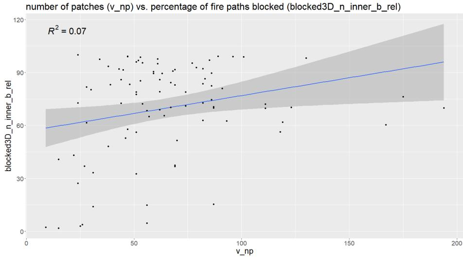
Figure D14: Metric of number of patches to the percentage of fire paths blocked.
