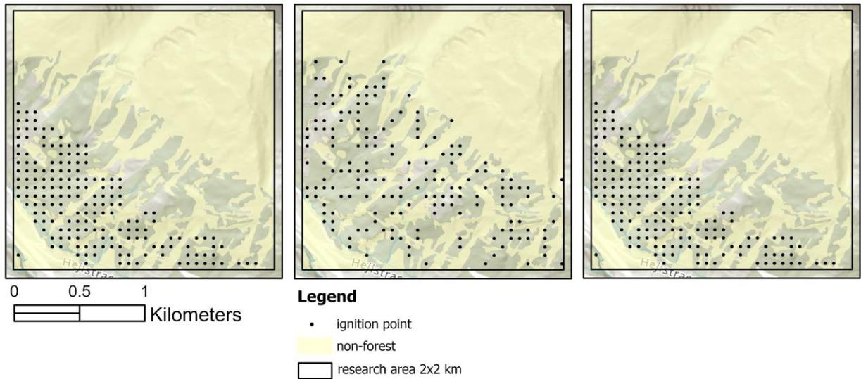
Figure 13: The three different methods for setting the ignition points which were tested. Left all ignition points within the forested area, extracted from grid intersections with distances of 65 m (= original). Middle randomly selected 50 percent of all ignition points from the original version. And on the right, 50 percent of the points (from the original version) at the lower altitude.
