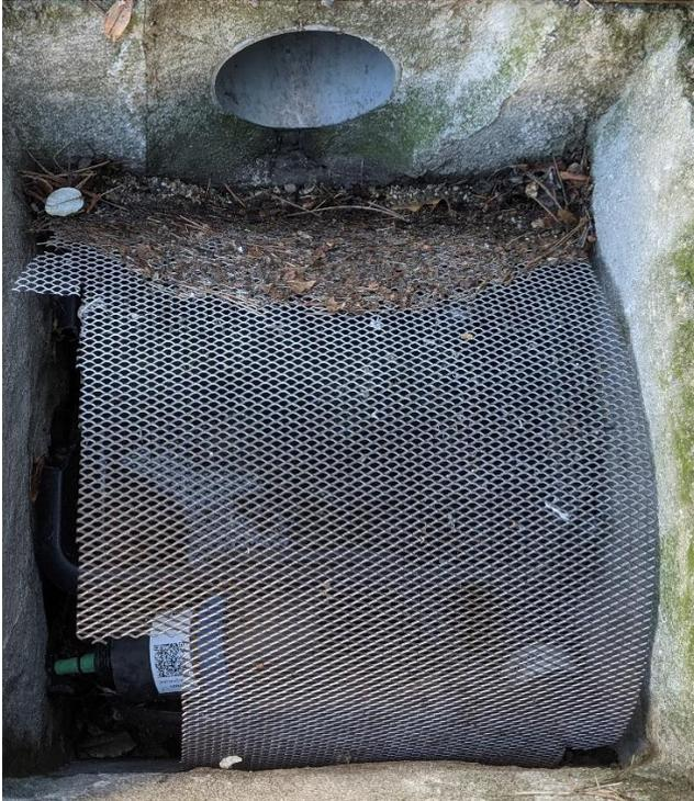
Figure 5: Surface runoff gauging station, covered with a protection rake.
