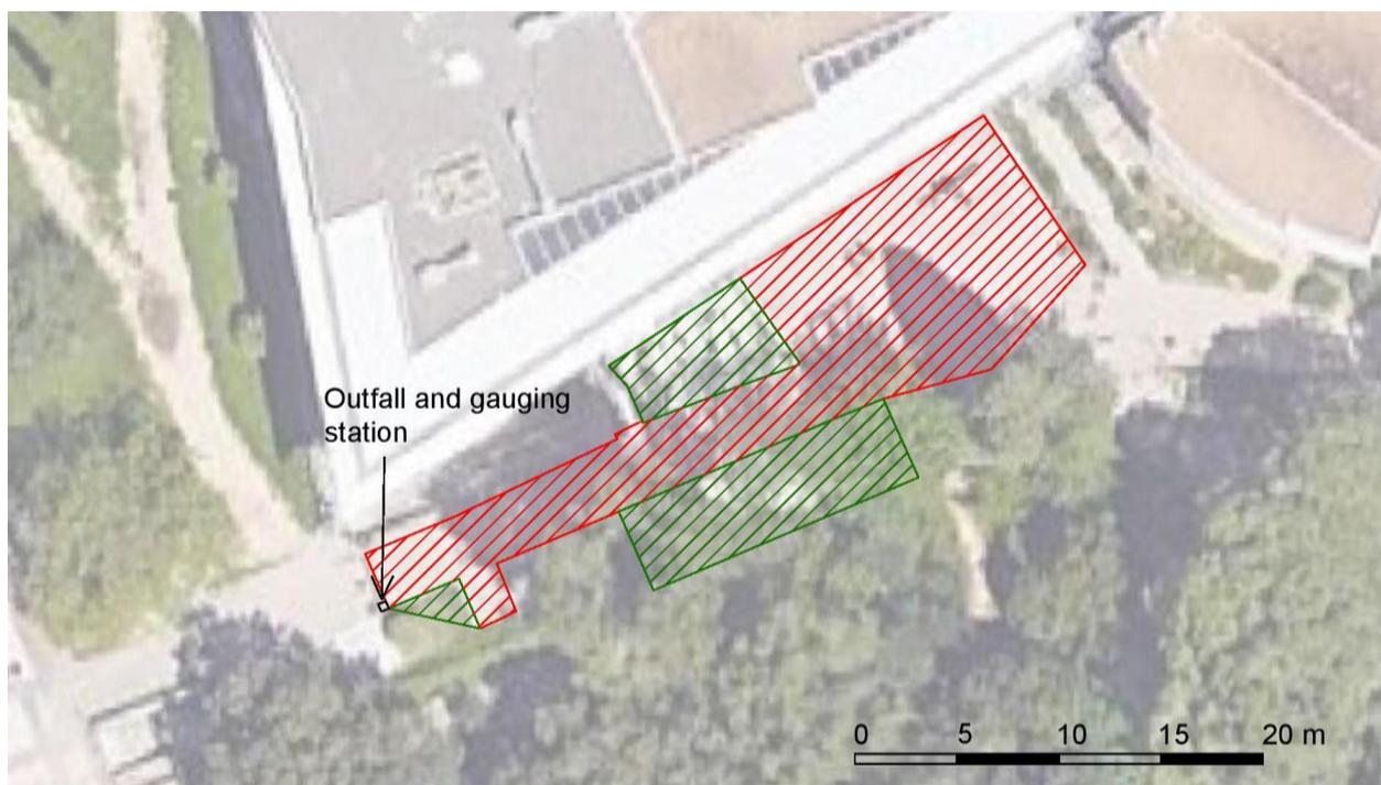
Figure 2: Study site “Polytech”, pervious surfaces are hatched in green, impervious surfaces are hatched in red.
