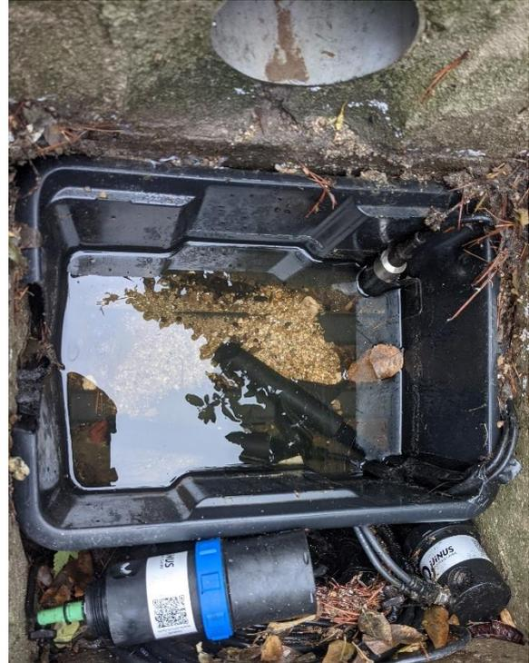
Figure 6: Surface runoff gauging station consisting of a sampling bucket with 3 sensors.
