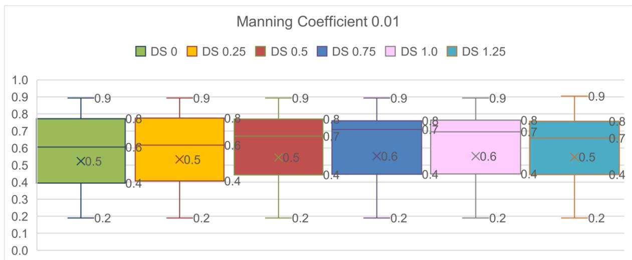
Figure 16: Boxplots which present the hydrological calibration results by combining all BFC efficiencies for different DS and a fixed  $n$  of 0.01.
