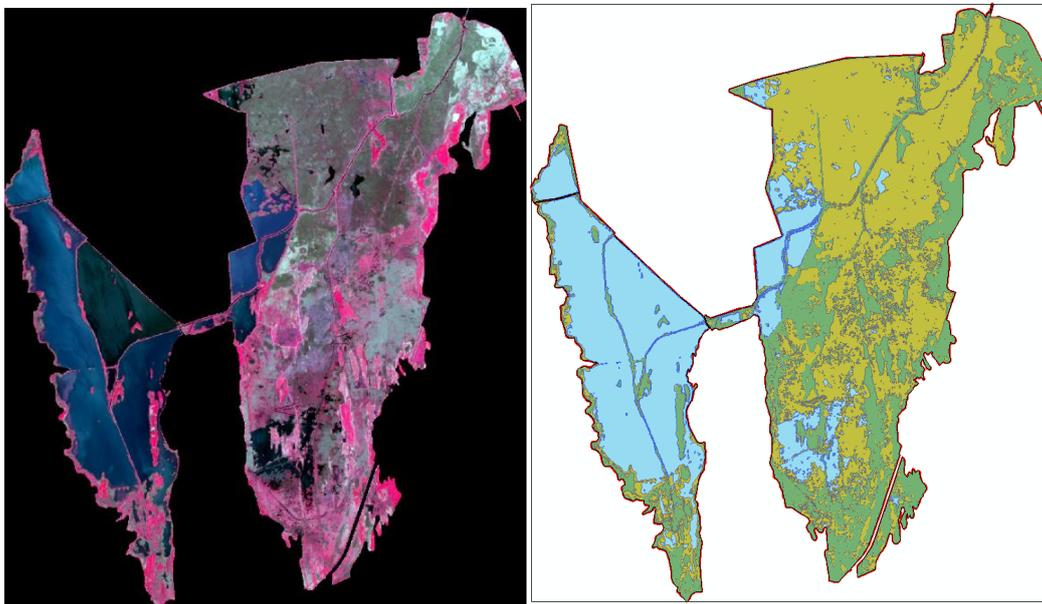
Figure 11: Left: Near-infrared image from Sentinel-2 satellite for 01.06.2022; Right: Clusterized map of the left hand-side image (blue: open water surface; yellow: reed; green: grassland)
