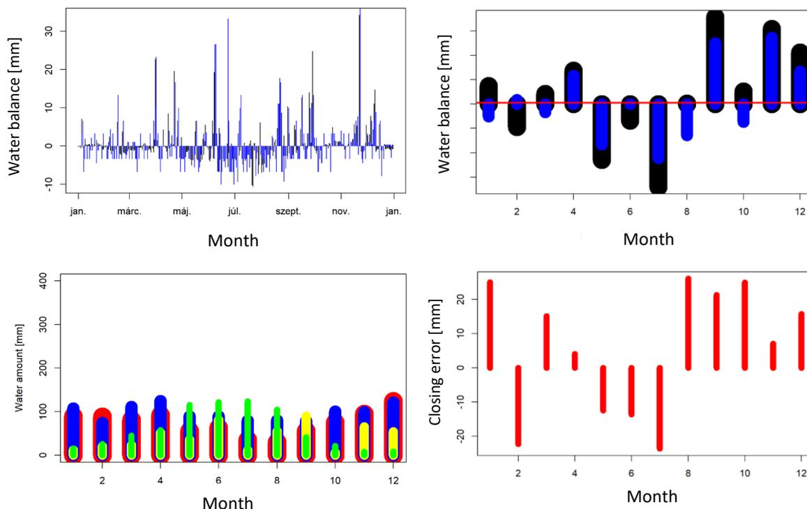
Figure 31: Water balance results of Ingói-pond; upper left: daily balance for 2022 [blue: storage change; black: calculated]; upper right: daily balance for 2022 aggregated to monthly values; lower left: input elements in the calculation for 2022 [blue: inflow, red: outflow, green: ETP, yellow: Prec.]; lower right: monthly closing errors in mm for the calculation
