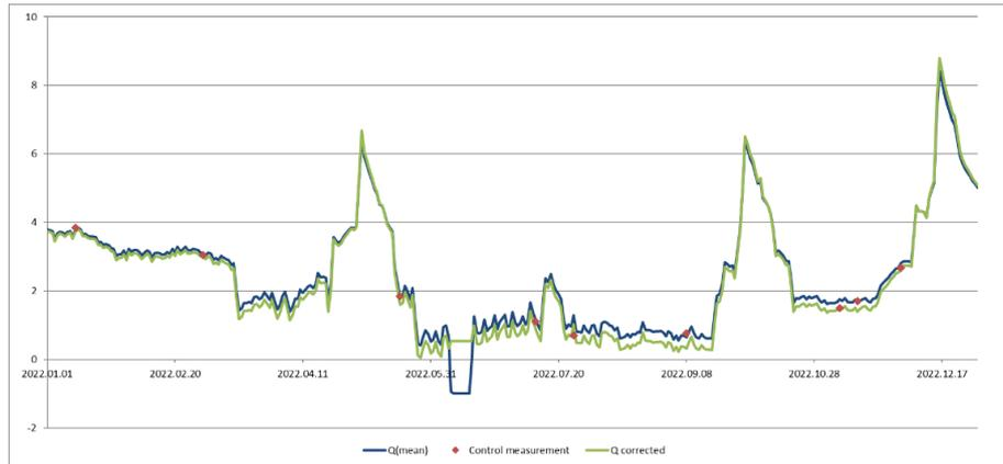
Figure 27: Original and corrected daily mean discharge time series for 2022 at Zala-Balatonhídvég station (x axis: Date, y axis: discharge in m<sup>3</sup>/s)
