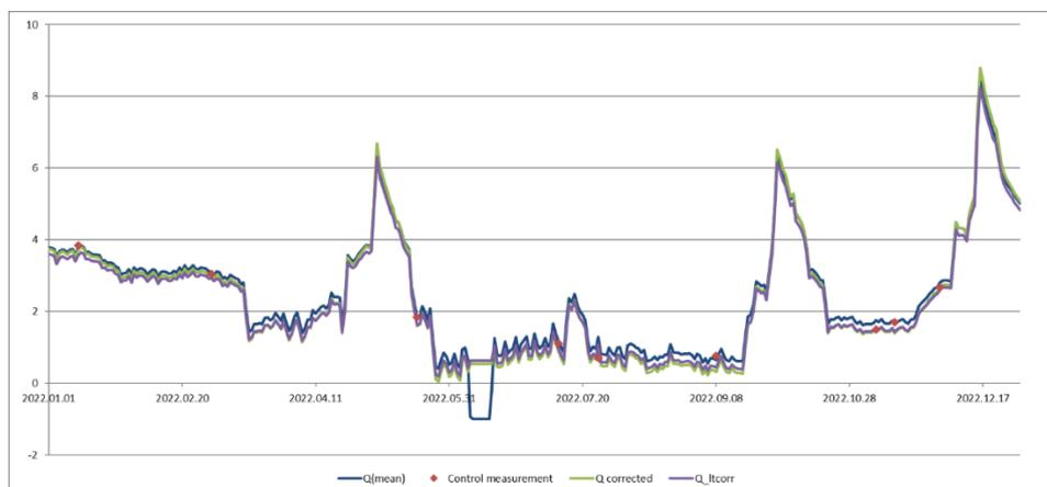
Figure 29: Original and re-corrected daily mean discharge time series for 2022 at Zala-Balatonhídvég station (x axis: Date, y axis: discharge in m<sup>3</sup>/s)
