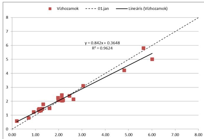
Figure 14: Correlation of automatically measured discharge (x axis) and control measurements (y axis) [m<sup>3</sup>/s]
