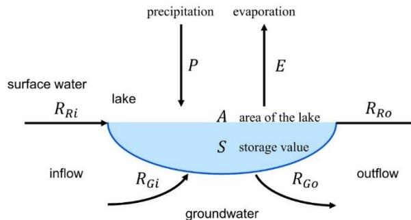
Figure 9: Elements of water balance in a lake (Water balance lake, 2019)
