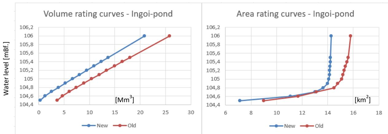
Figure 40: Old and new volume and are rating curves for Ingói-pond
