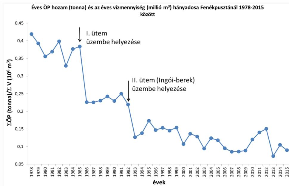
Figure 3: Total phosphorous load in the mouth section of Zala between 1978 and 2015. The arrows indicate the starting of operation of the I. phase (Hídvégi) and the II. phase (Ingói) (NYUDUVIZIG)
