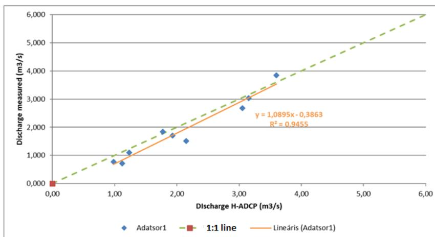
Figure 26: Correlation of automatically measured (H-ADCP) and control discharges at Zala - Balatonhídvég station, 2022
