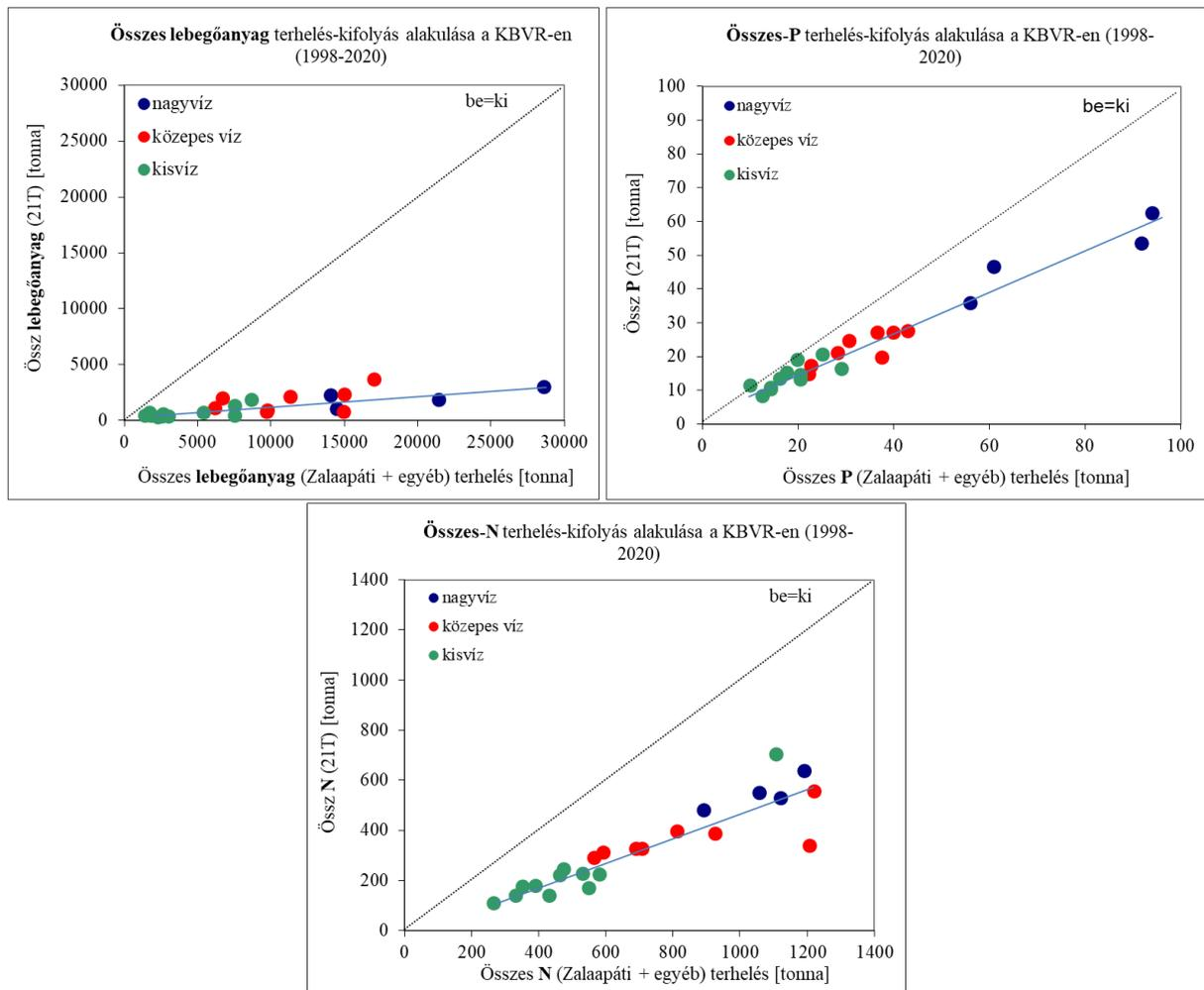
Figure 6: Ratio of the inflow and outflow of TDS, TP, TN loads in the Kis-Balaton system; horizontal axis: inflows, vertical axis: outflow. The blue dots refer to floods and high-water situations, the red dots refer to mean water and the green dots refer to low water conditions. (Department of Water Protection and Watershed Manag, 2021)
