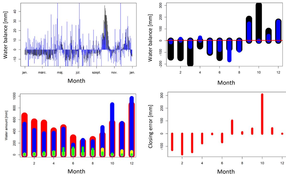
Figure 41: Water balance results of Fenéki-lake; upper left: daily balance for 2022 [blue: storage change; black: calculated]; upper right: daily balance for 2022 aggregated to monthly values; lower left: input elements in the calculation for 2022 [blue: inflow, red: outflow, green: ETP, yellow: Prec.]; lower right: monthly closing errors in mm for the calculation
