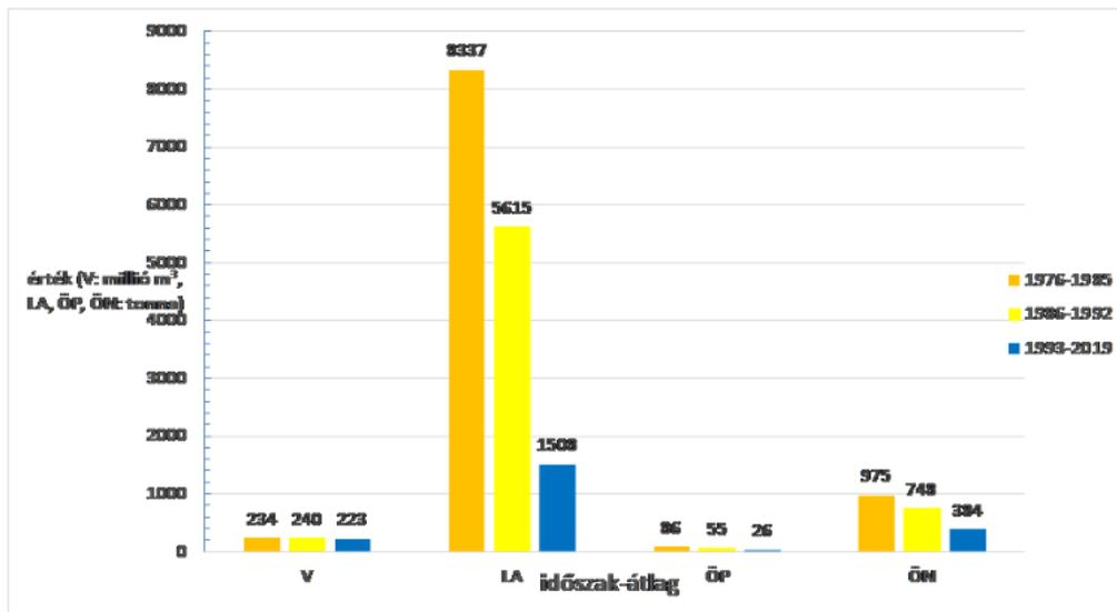
Figure 5: Mean Discharge volume (V), mean TDS load (LA), mean TP (ÖP), mean TN (ÖN) at the mouth section of Zala River in different periods (orange: 1976-1985; yellow: 1986-1992; blue: 1993-2019) (NYUDUVIZIG, 2022)
