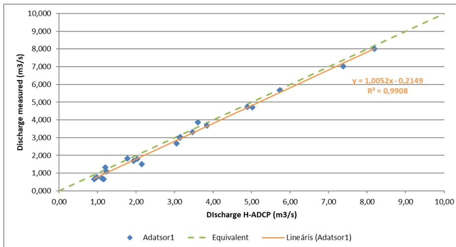
Figure 28: Correlation of automatically measured (H-ADCP) and control discharges at Zala - Balatonhídvég station, 2020-2022
