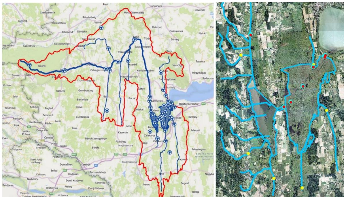
Figure 8: Left: Overview of automatized stations on the Kis-Balaton catchment (source: WebSCADA telemetry system); Right: Discharge measuring stations across KB (Red dots: Automatized; Yellow dots: Rating curve method and occasional measurements)
