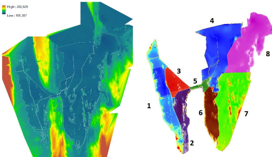
Figure 12: Left: DEM based on Lidar and sonar survey (units: mBf.); Right: Splitted parts for new rating curves
