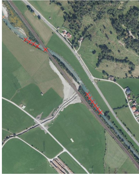
Figure 45: Not fishpassable instream barriers within 50 metres from railway infrastructures
