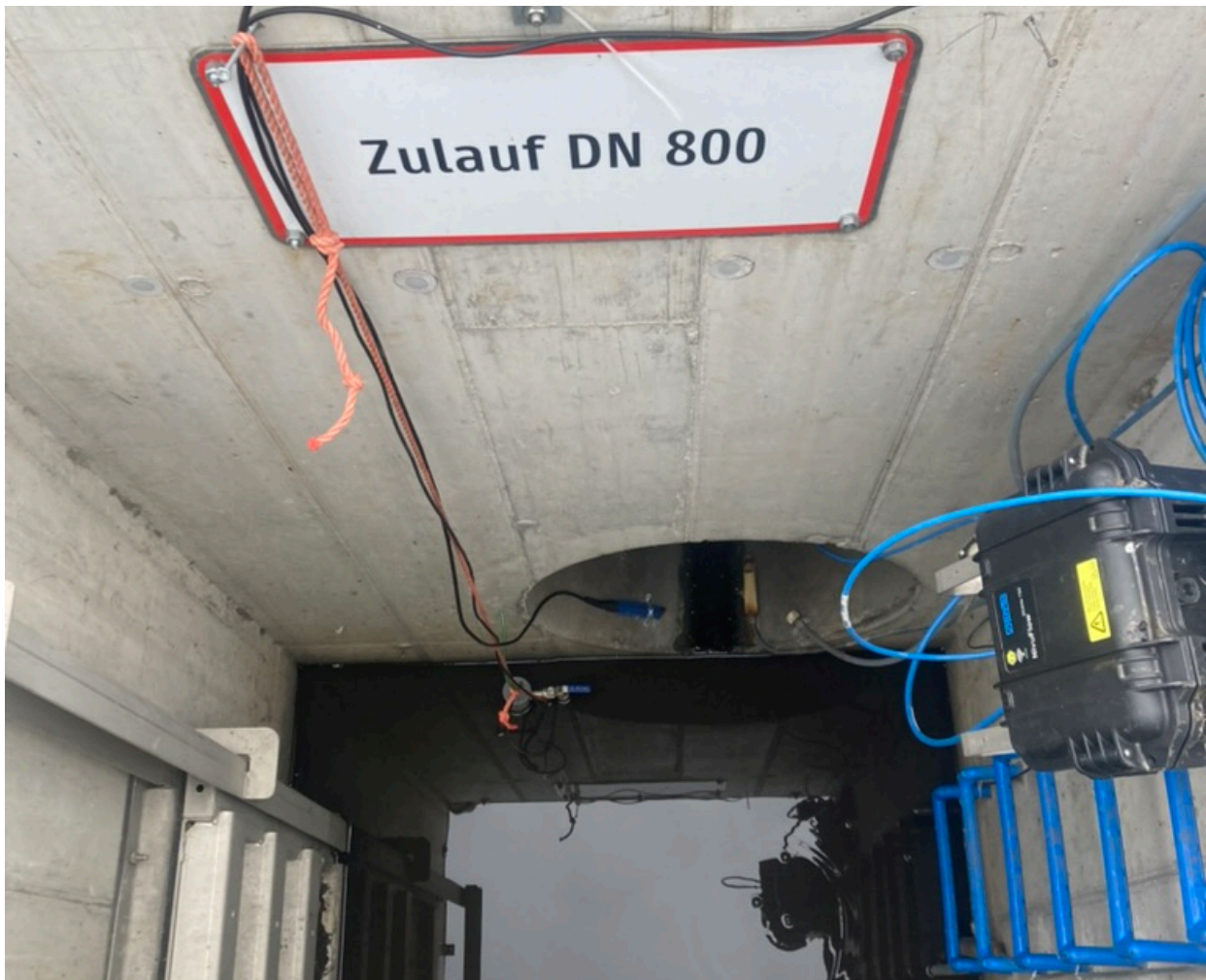
Figure 5: Influent pipe where the automatic sampler takes water samples and where the nivus device takes measurements and shaft area where the total sampler is placed (attached to the orange rope)
