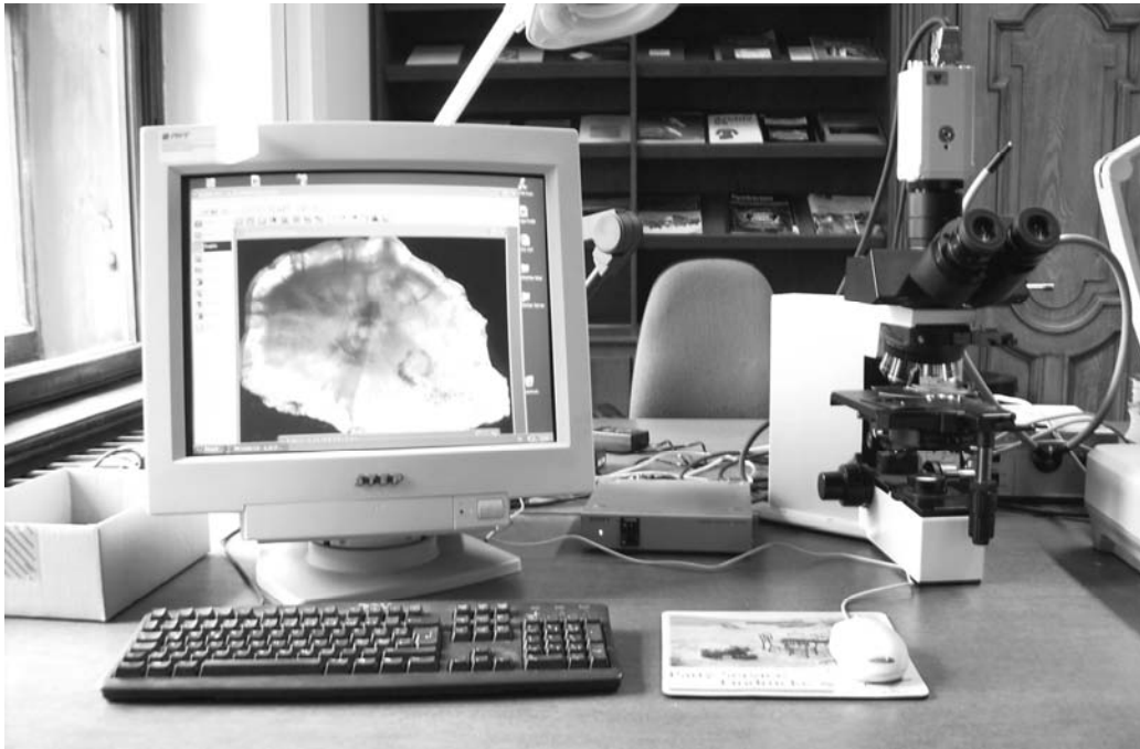
Figure 19. The digital imaging system KS 300 3.0 (Carl Zeiss MicroImaging GmbH, Göttingen, Germany) in combination with a light microscope (Olympus BX 50, Olympus Europa GmbH, Hamburg, Germany), a camera (Sony Power HAD 3ccd Color Video Camera, Sony Corporation, Tokyo, Japan) and a camera adaptor (Sony Camera Adaptor CMA-D2, Sony Corporation, Tokyo, Japan) at the Museum of Natural History, Vienna, Austria.
