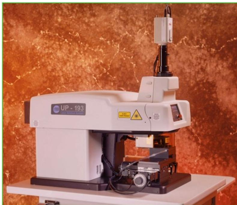
**Figure 3.** The UP193 Solid-State laser ablation system [New Wave research 2005].
