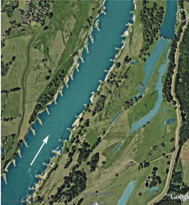
**Figure 2.12:** A sequence of backward inclined groynes at the river Elbe near Havelberg, Germany (image: Google earth).
