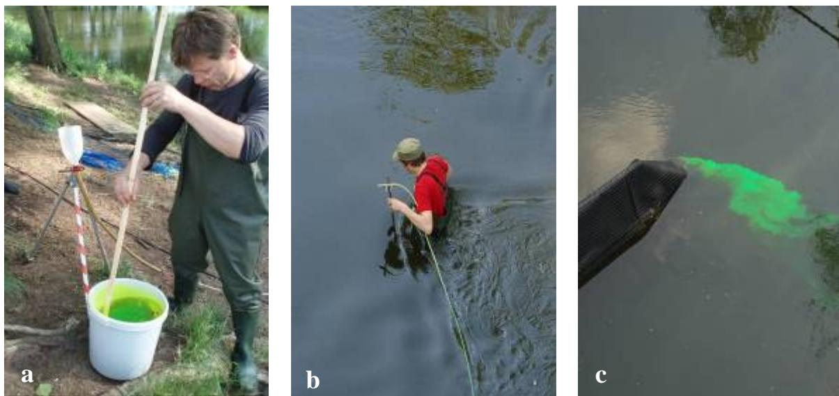
**Figure 3.23:** Dye injection: Dissolving of uranin dye (a), fixing of the injection tube (b), and injection (c).
