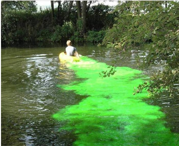
**Figure 3.21:** Dye injection for tracer studies: uranin dye injected as a line source across the river (river Spree, 2007).
