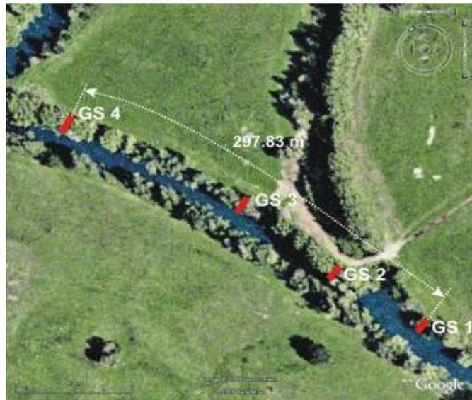
**Figure 3.24:** Experimental river reach with gauging stations (GS) 1 to 4 at the experimental river reach (river Spree, 2007).
