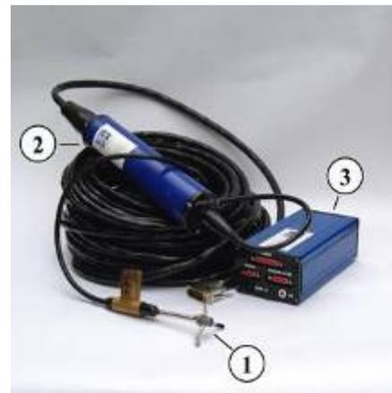
**Figure 3.11:** Nortek Doppler Velocimeter NDV employed for field measurements at the river Spree, 2007
