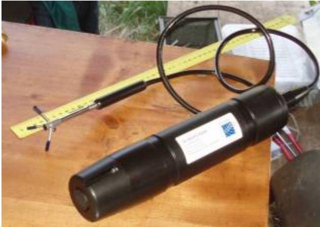
**Figure 3.14:** NorTek Vectrino Doppler Velocimeter employed for field measurements at the river Spree, 2007.
