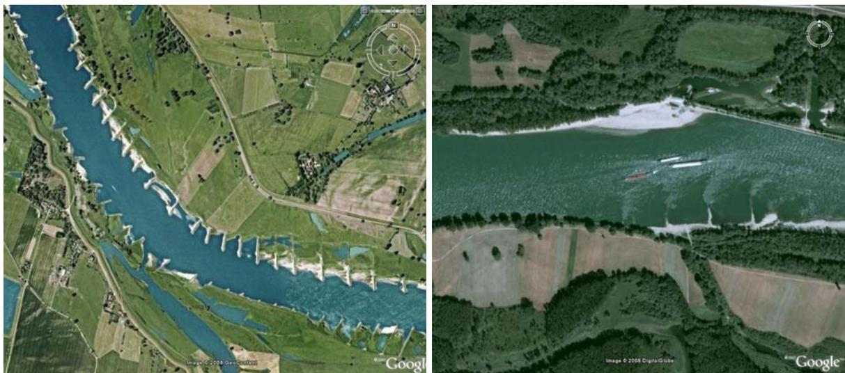
**Figure 1.1:** Airborne photos of groynes at the river Elbe close to Wittenberge, Germany and the at river Danube downstream of Vienna, Austria (images: Google earth)
