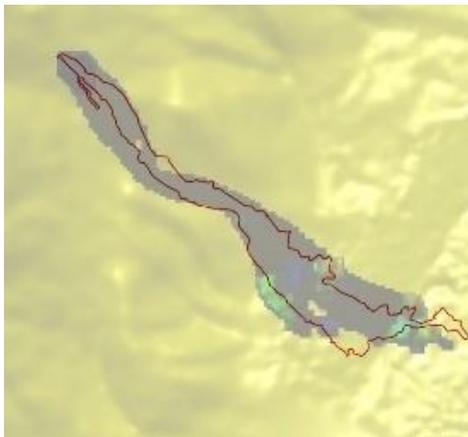
Figure 26. *The 1990 Tsing Shan debris flow: Model predictions versus Field observations*
