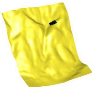
Figure 12. *SPH mesh to model a debris flow in Hong Kong*
