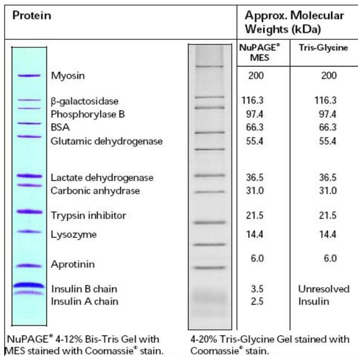
**Figure 3-6: Approximate molecular weights of the protein bands from the molecular weight standard Mark 12 (Invitrogen)**
