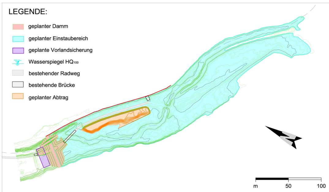
Figure 16.4: Overview of the retention measures at flow kilometer 2,550 including the planned water storage area, based on IBL (2009)
