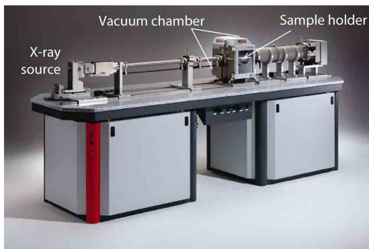
Figure 23: The device used for obtaining the 2D-WAXS x-ray diffraction patterns, a Bruker AXS Nanostar system. The radiation was produced with a rotating anode generator with a Cu target (not displayed). The samples were put in a vacuum chamber. Wires for applying the electrical field were put in a gas tight feed through. (Image from a Bruker presentation, (Bruker AXS, 2009))
