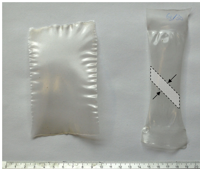
Figure 20: Cellulose-films before and after stretching. This sample is a cellulose-film with 6 g cellulose. The dotted line shows how the Piezo specimens were cut out of the dried and stretched foils. (Scale in centimeters)
