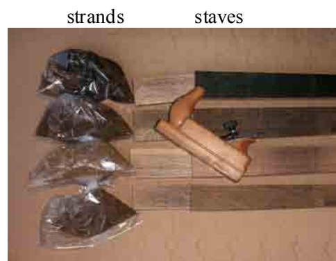
Figure 2: Oak staves: four different toasting variants (Heavy, medium plus, medium long and light)
