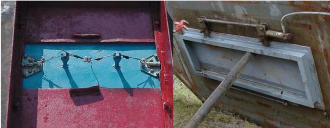
**Figure 57:** Mechanism of slot cover (Bergman et al., 2007) compared to mechanism of trap door
