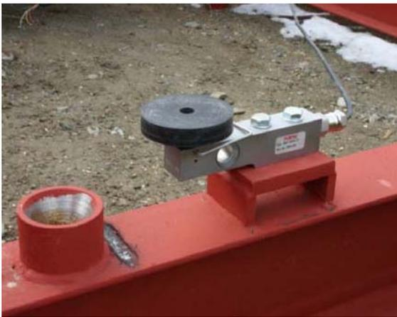
**Figure 31:** Close-up view of deployed load cell
