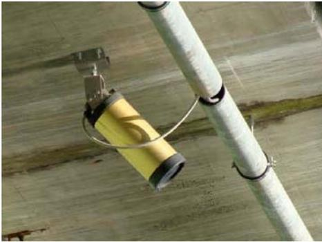
**Figure 8:** OTT-radar sensor
