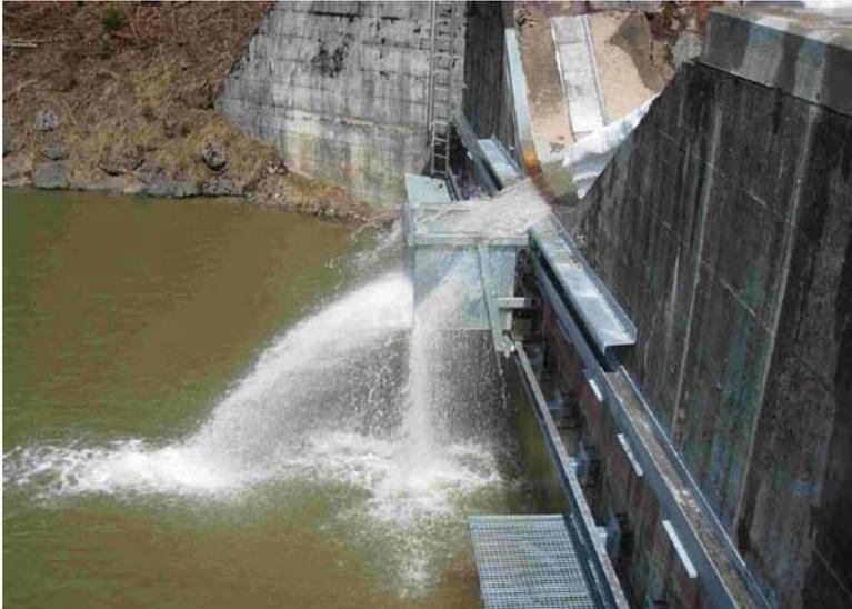
**Figure 62:** Basket trapping bedload sample (Rickenmann et al., 2010)
