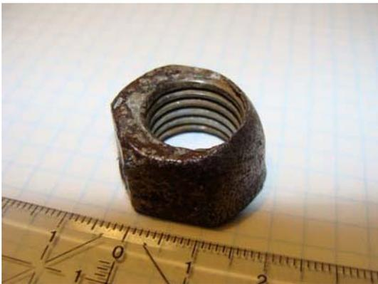
**Figure 38:** Worn out M16 screw nut after one-year operation
