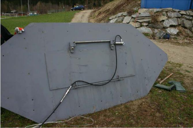
**Figure 35:** View of the under-side mechanism of the slot door
