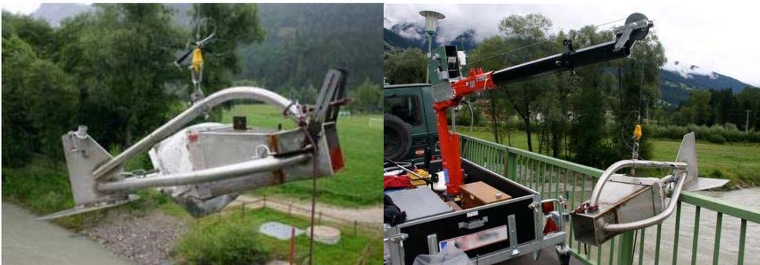
**Figure 11:** Large HS sampler & trailer with mounted cable winch
