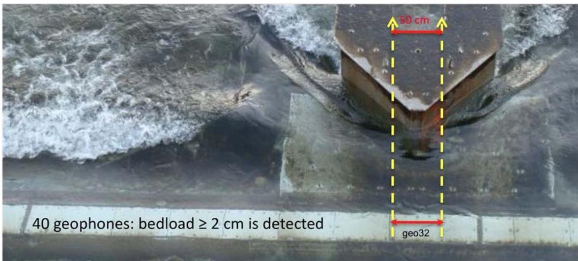
**Figure 20:** Location of lift trap in relation to geophone device
