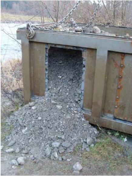
**Figure 58:** Faulty removal of the trap side door
