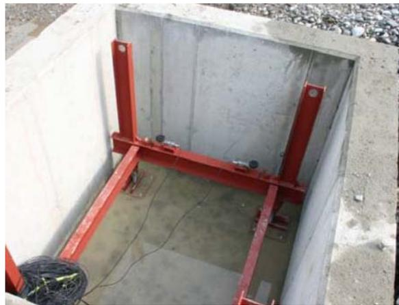
**Figure 32:** Arrangement of load cells in fixed slot trap
