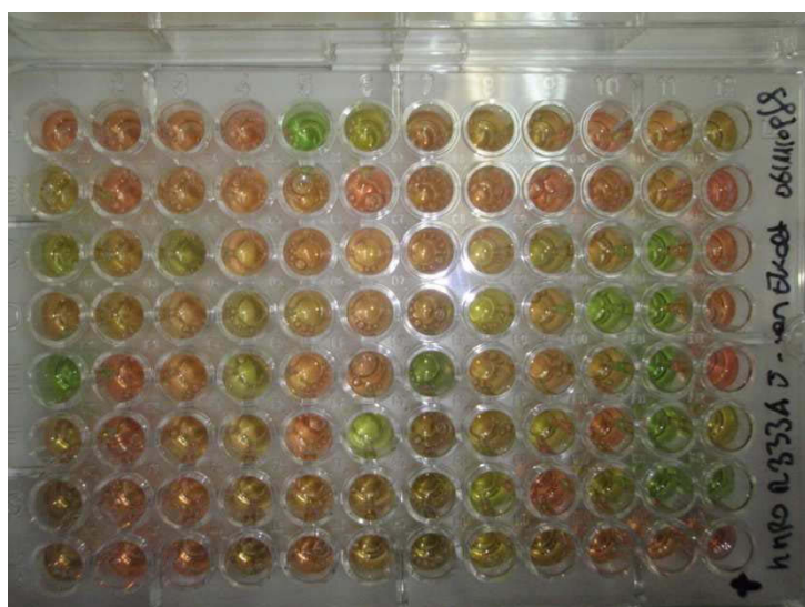
Figure 3-2: example for ABTS screening in a 96-well plate
