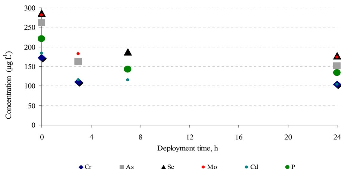
Figure 5.5.1. The concentration of the experimental solution after different times of deployment. The values at the Y axis show the initial concentration of the solution before exposure of the DGT device.
