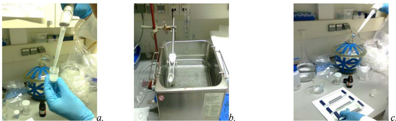
***Pictures 4.2.1.: a. A pipette was used for mixing the La-Chelex resin with the viscous gel solution; b. An ultrasonic bath was used for mixing the powdery mineral resins with the viscous gel solution; c. Glass plates were used to prepare DGT resin gels.***
