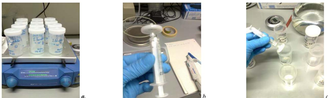
**Picture 4.7.1.:** a. The DGT resins gel discs were shaken during deployment; b. and c. Syringe filters were used to filter the immersion solution
