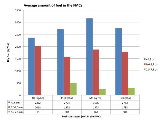
Figure 11: Average amount of fuel per size class [dry kg/ha], in the FMCs: TH, PL and MR.
