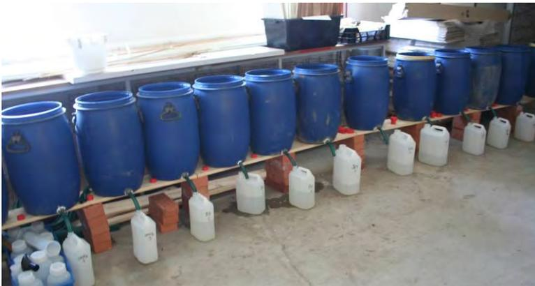
Fig. 1: Experimental set-up of the wood ash leaching experiment in barrels
