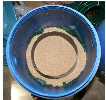
Fig. 2: Ring for water distribution and top layer of silica sand
