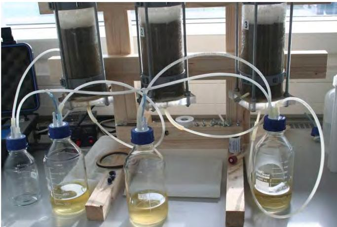
Fig. 3: Experimental set-up of the soil column experiment
