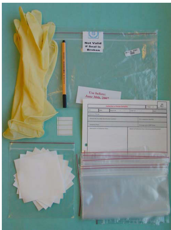
Fig. 1.1-1: Cotton swipe sampling kit (adopted from (Zendel et al., 2011)).
