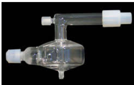
Fig. 1.5-2: Quartz cyclonic spray chamber. The figure was adopted from (Elemental Scientific. Cyclonic Spray Chambers.)
