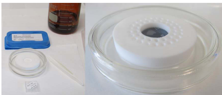
Fig. 5.1-1: Particle transfer onto a cellulose acetate membrane.
