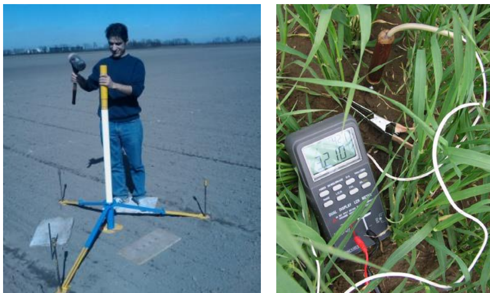
Fig. 8: Installation of PVC access tubes for capacitance probe and measurement of root electrical capacitance
