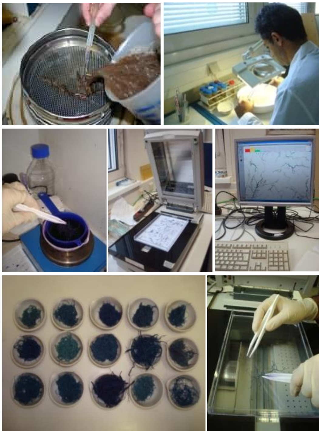
Fig. 7: Preparing roots for image analyzing: (i) washing, sieving and separation of roots; (ii) staining with Giemsa solution (azur-eosin-methylenblue); (iii) scanning and image analysis; (iv) individual stained root samples
