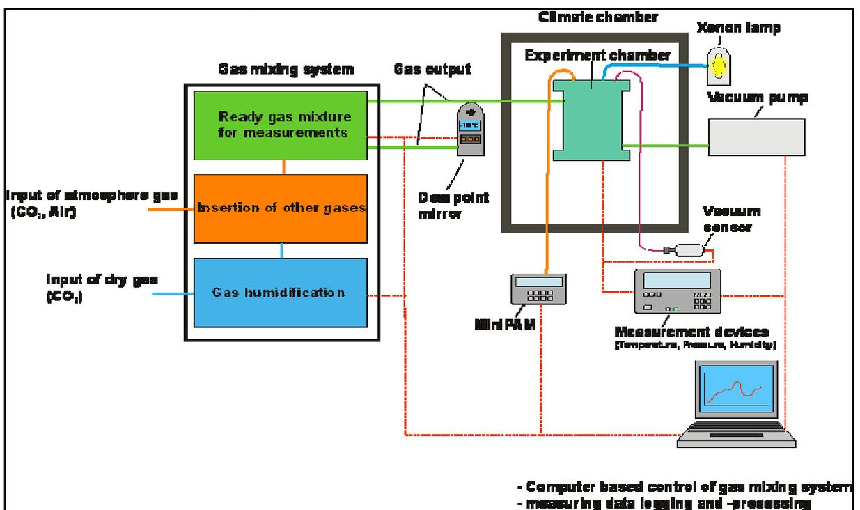
Figure 6. Scheme of Mars Simulation Chamber (provided by Lorek A. and de Vera J-P)
